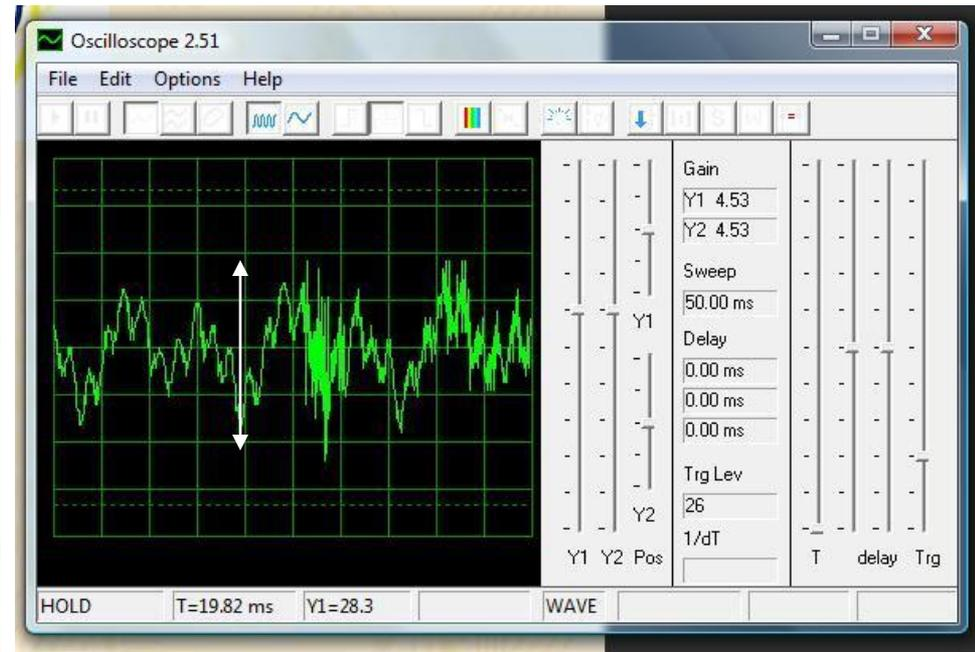
Constant Sound is now produced by the Signal Generator. The signal drives a Toy speaker from the Snap Kit. The sound is picked up by a microphone and the waveform is displayed via the Winscope Program available also from the Snap Kit. Please compare this with the next slide.
