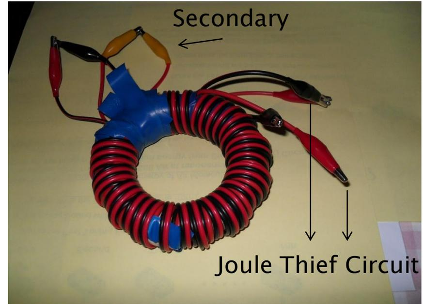
The Prototype under test was produced by Mr. Michael Du in Irvine USA. The Air-core Toroid with two secondary windings was used. The Input is from the battery side of the Joule Thief. The Output is from the yellow clips of one of the two secondaries. The instantaneous values were displayed.
