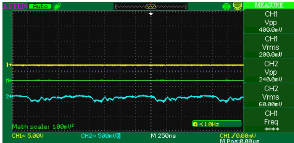
This comparison is between the Input of a Joule Thief circuit and the Output from a Secondary winding on the air toroid.
