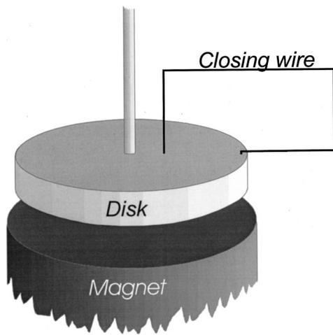
Fig. 1. Faraday's setup: magnet, disk and closing wire.
