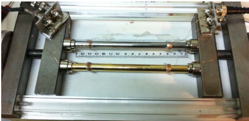
Figure 5. Magneto-acoustic test rig with the two Permendur rods
