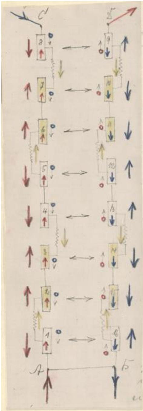
The yellow arrows show the direction of the extra currents and the corresponding charged plates. The pencil arrows with the colored circle show the current path of the predominant current caused by the closure of A B, the colored arrows next to the plates the current direction in the flat coils above the plates, the colored arrows finally in the plates, the resulting basic current direction by opening A B.
