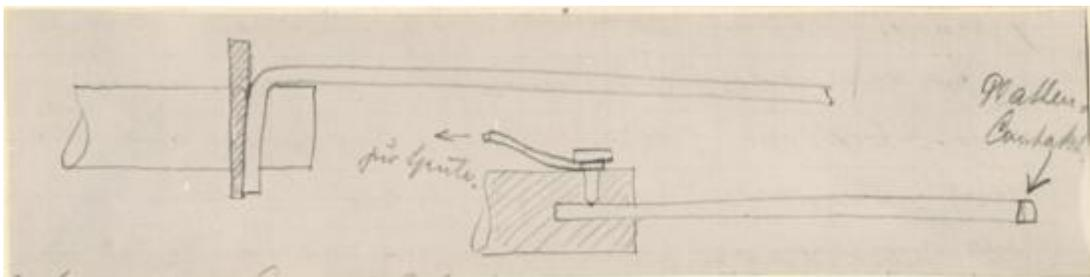
Any other construction is equally suitable, provided it achieves intimate contact between tungsten steel and iron. The latter construction is much easier since it achieves a galvanic connection of the core with the corresponding plate, making the permanent magnet act as a conductor between the core and plate.
