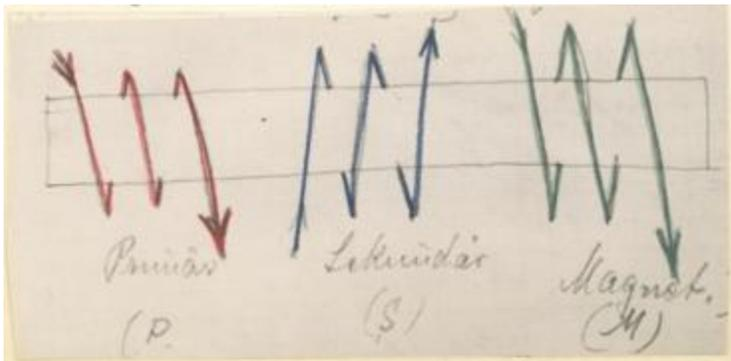
The half of the required magnets on the left, the other half on the right. The former have a north pole at the primary and magnetic coil entrance, a south pole at the exit, the latter a south pole at the entrance and a north pole at the exit. In the secondary coil, it is reversed.
