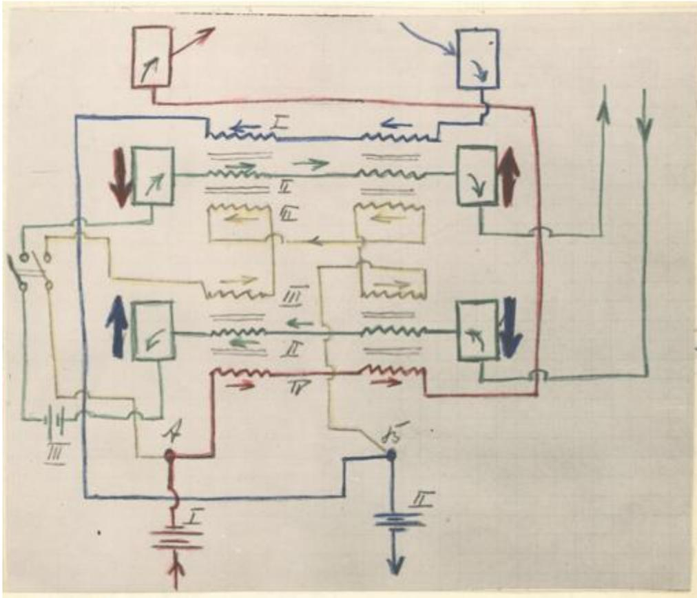
13. The mode of operation is now explained. First, it should be emphasized that the cores used in the interrupter are not permanent magnets but made of soft iron, as shown by the following considerations.
