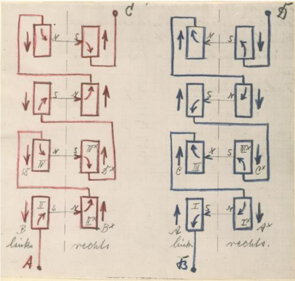
The blue and red arrows next to the plates indicate the direction of current in the flat coils above the plates, the arrows in the plates indicate the direction of the plate current when A B is opened.
