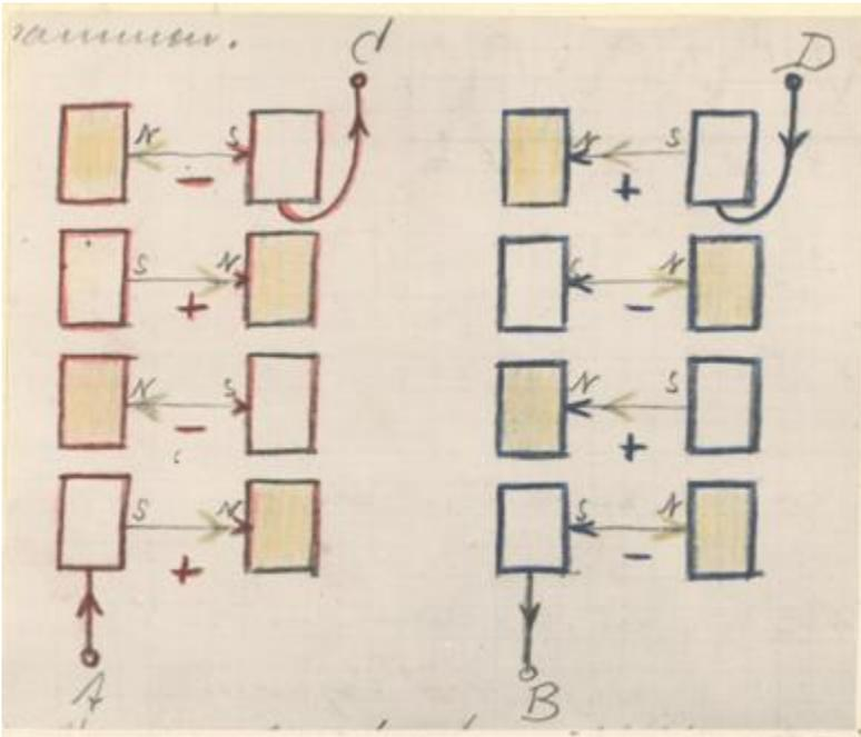
When the magnetic field disappears, as known, extra currents are induced in the direction of the yellow arrows and charge their energy into the yellow-shaded plates. When the field reappears, the opposite extra currents occur and charge the other capacitor plates accordingly.
