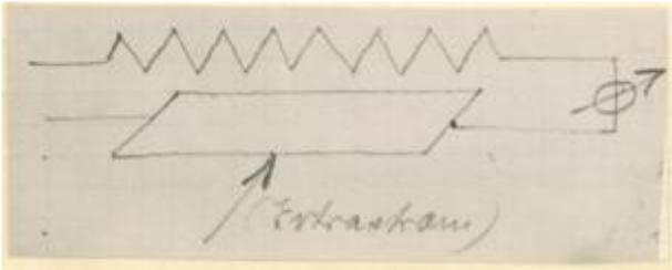
When the flat coils are completely turned off, a current flows between them and the plates above and below when an extra current enters the plate.
