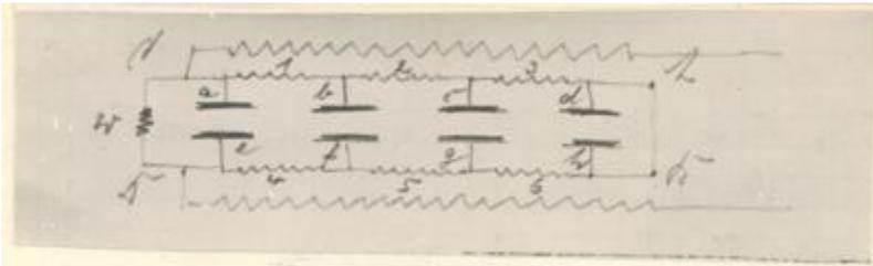
Of fundamental importance here is the well-known phenomenon that when switching off DC magnets very quickly (as is the case in my apparatus), the magnetic energy is largely converted into electrostatic energy, and high overvoltages arise, which can endanger the insulations under certain circumstances.
