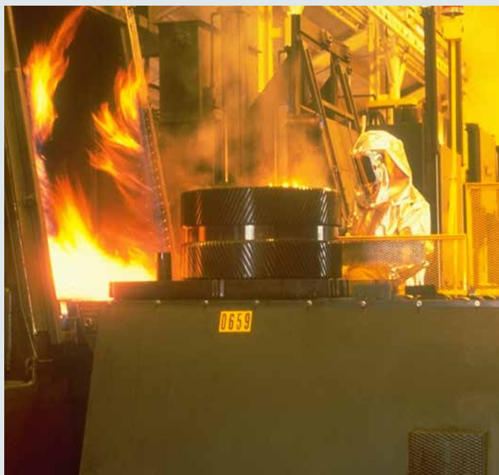
Figure 1: Atmosphere gas carburizing
