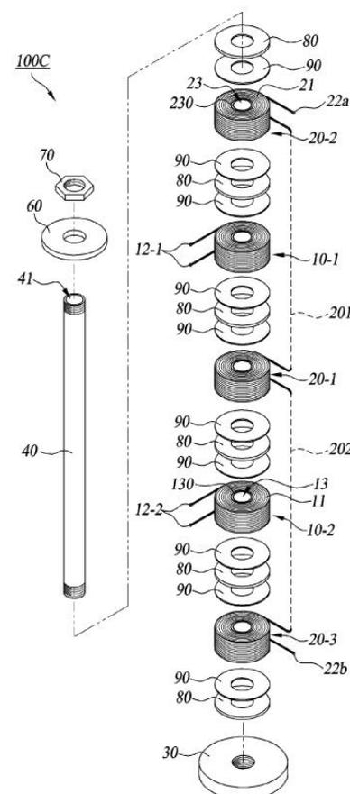
**Figure 6. Core and coils**
