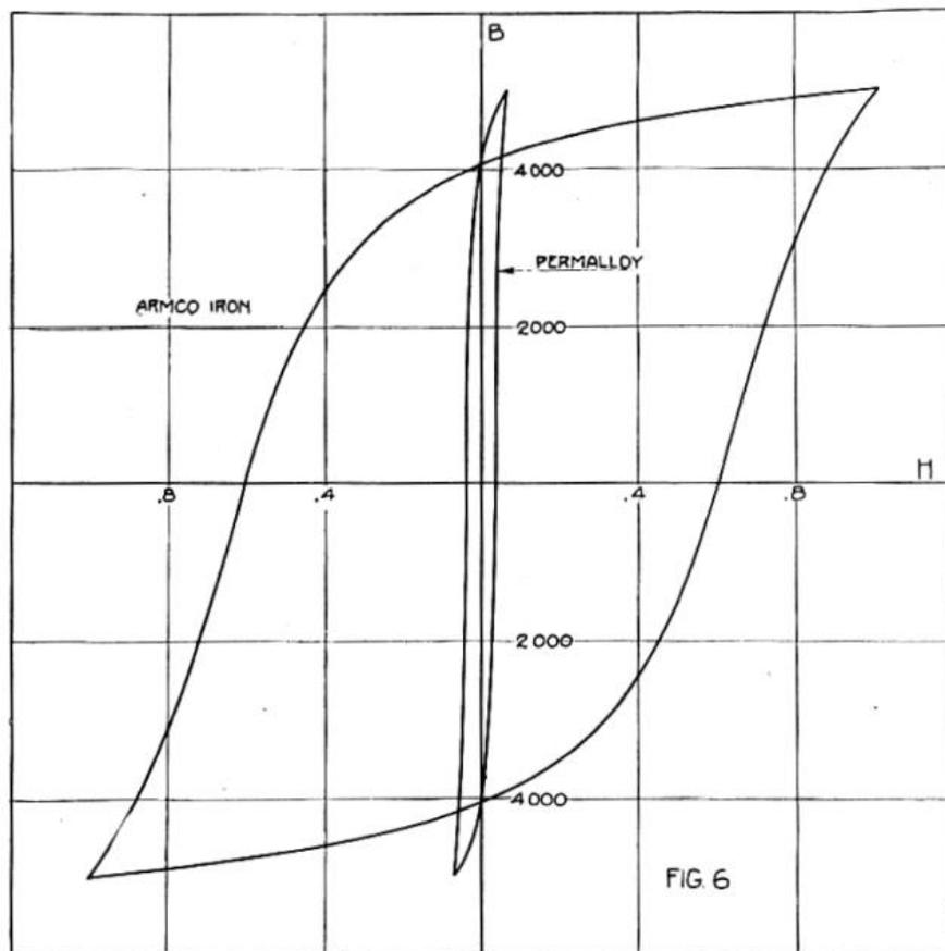
**Figure 9. BH loop for Armco iron**
