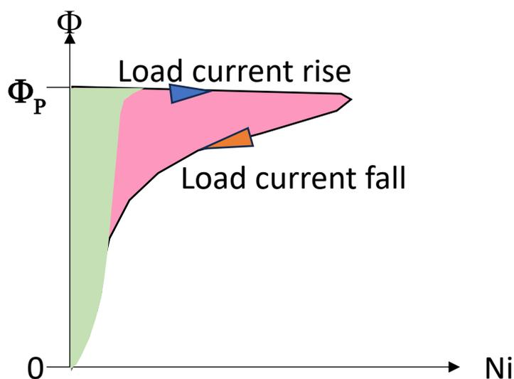
**Figure 4. Expected demagnetizing curve.**
