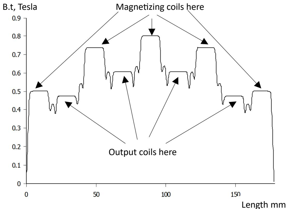
**Figure 8. Flux density along the core**
