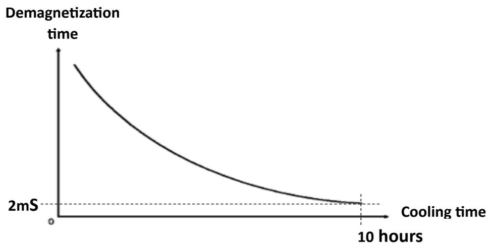
**Figure 5. Demagnetization time v. cooling time**
