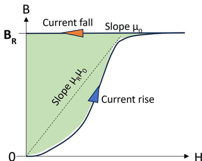
**Figure 1. BH curve for magnetizing pulse**
