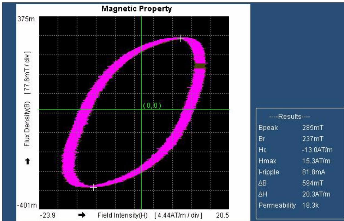
Above shows BH curve for unloaded composite primary (P1 and Ret1)
