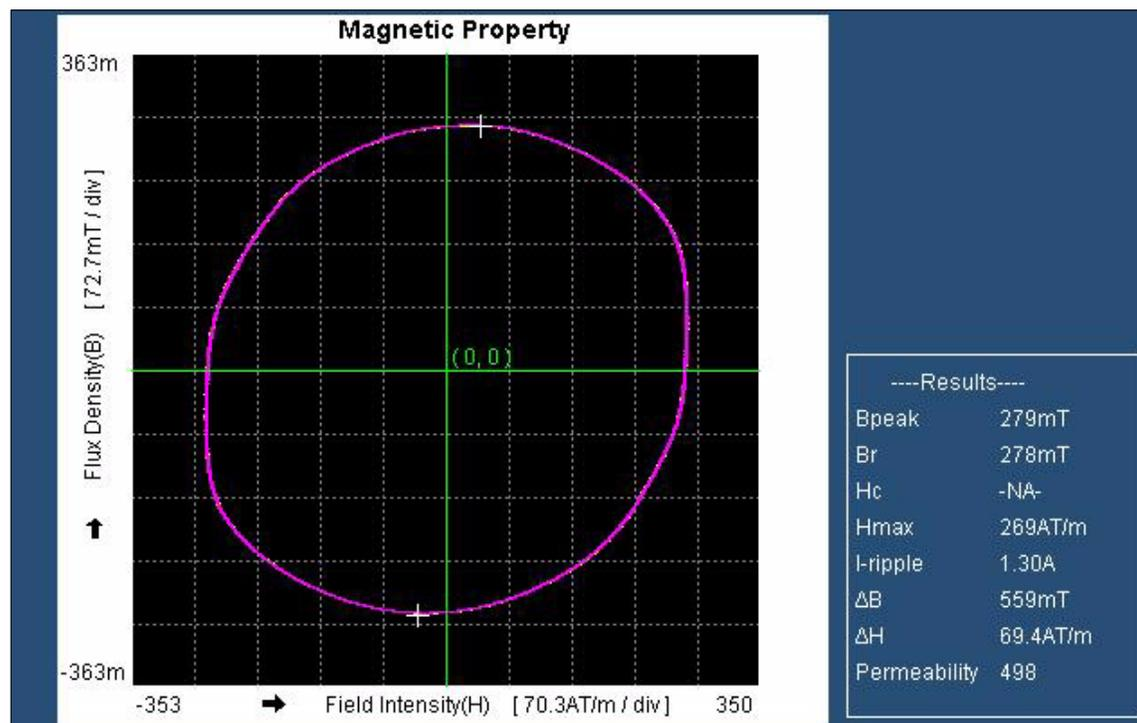
Above shows loaded BH curve again measuring composite primary.
