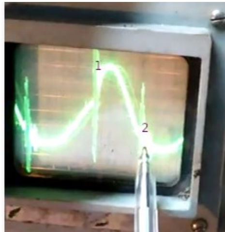
1 – MOSFET open, 2 – closed (current trace)
