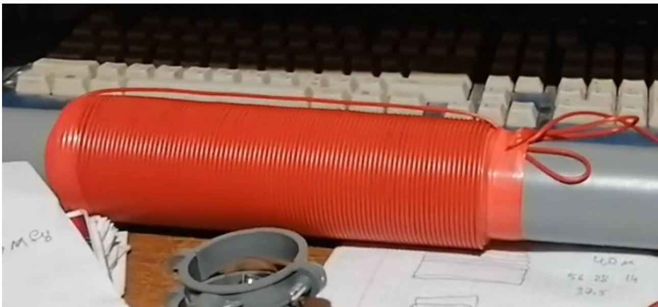
pic. 3 layer coil, resonance frequency 333khz
