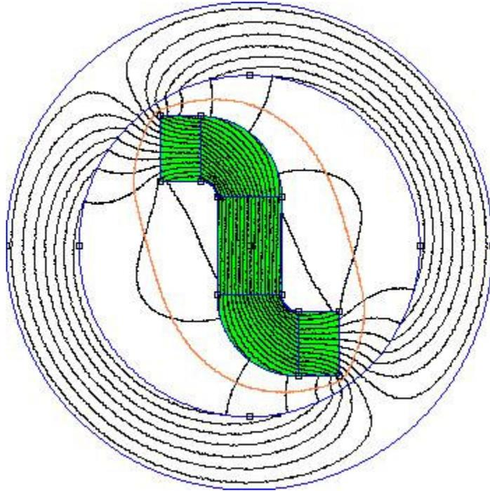
In fact FEMM draws a number of contours around the object as shown in the expanded image below, and integrates around them all. The black dots show the grid size used that in this case was 0.1mm.
