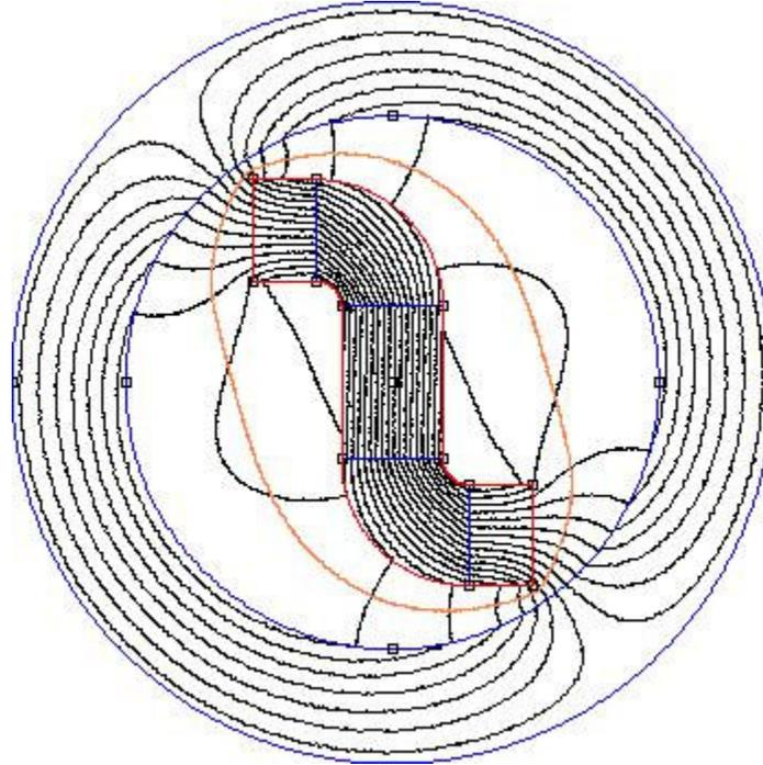
The CW direction for selecting the line contour is important because the material boundary is a discontinuity for the magnetic H field used in the tensor calculation, so FEMM uses a contour line slightly to one side of the delineated boundary, and that CW direction ensures that the contour is in the air space outside the object, and not within the object (this is all explained in the manual).
