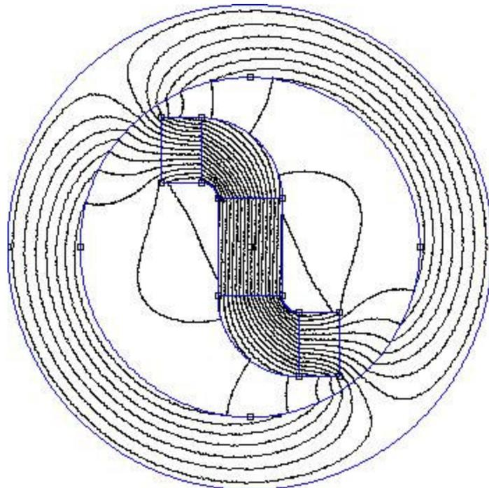
The interesting thing about the FEMM simulation is that it predicts a torque. Now you can obtain the torque by two different methods, both of which use the Maxwell stress tensor. The method recommended in the FEMM manual uses a stress tensor contour that is drawn around the object under consideration, you simply select the block whereupon it turns green, then select the torque integral function. FEMM draws its own stress tensor contour as shown orange in this image.
