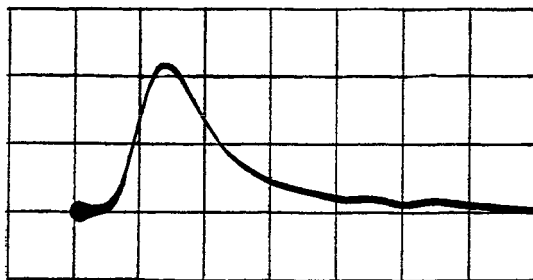
Figure 1. Photopulse illuminating the cathode; time base 10 nsec/div.
