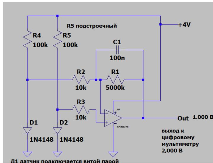
text: R5 is trimer, D1 thermal sensor, connected with twisted pair, output to digital multimeter 2V
