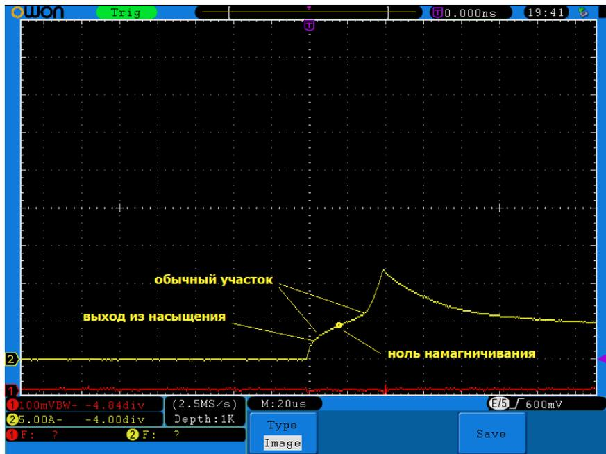
text: exit from saturation, normal region, zero magnetization
