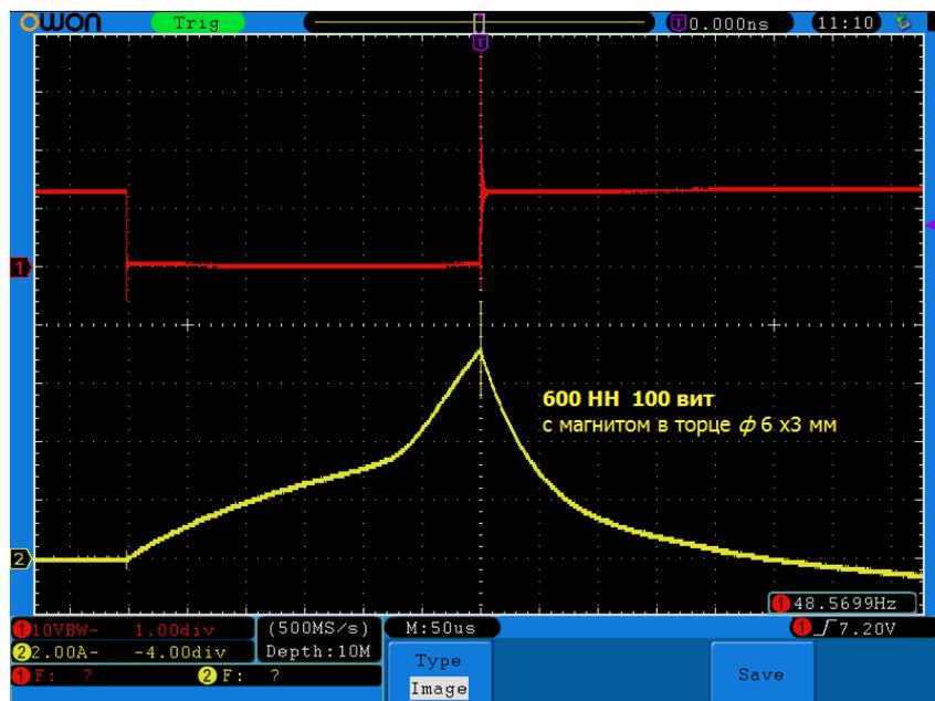
yellow text: ferrite rod diameter  $\mu=600$  100 turns magnet 6mm x 3mm attached to the rod edge
