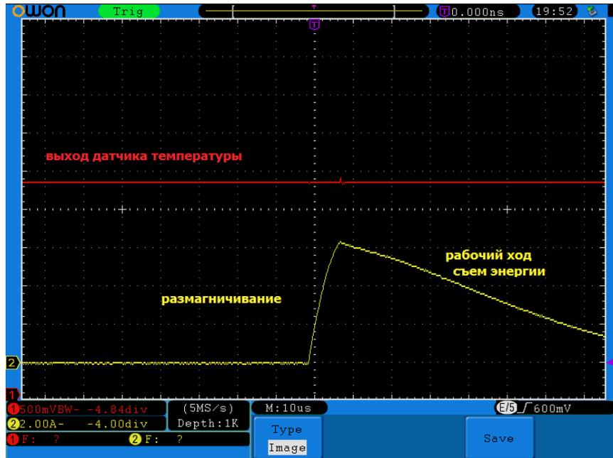
text: temperature sensor output (red), demagnetization (yellow), working region, energy pickup
