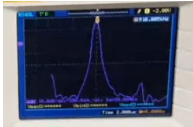
pic.2 first peak 910Khz
