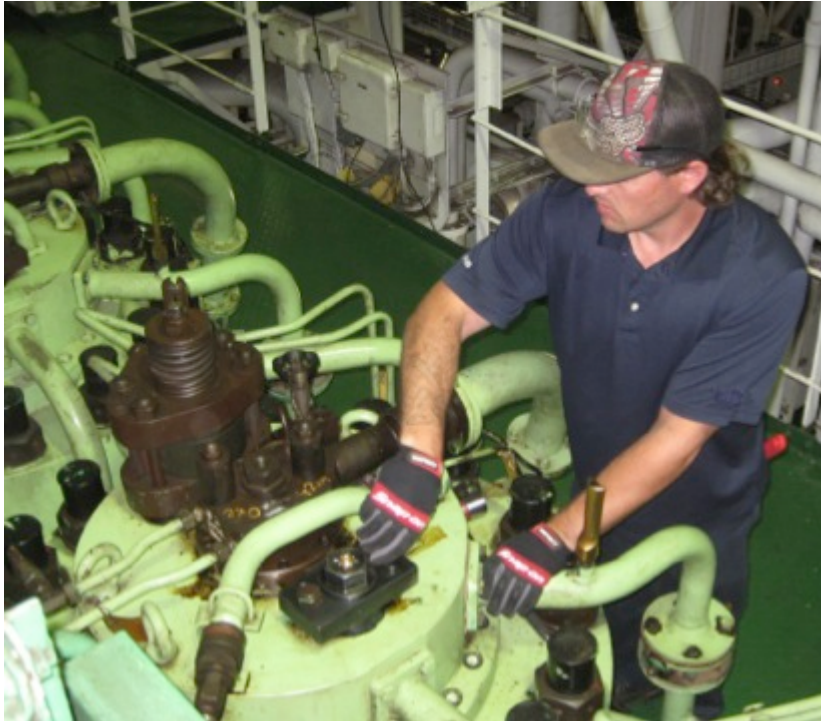
Photograph of TP relief valve being inserted into cylinder of Sulzer 6RND engine aboard MARAD vessel.
