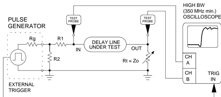
$R_g$  = GENERATOR SOURCE IMPEDANCE = 50 OHMS
