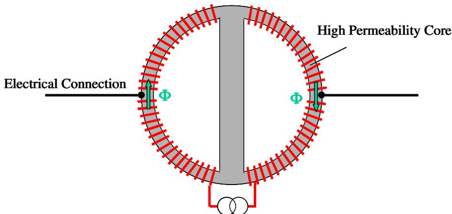
Finally we wind another coil on the central limb which when energized creates flux  $\Phi_c$  that adds to the core flux on one side and subtracts on the other. We thus achieve the objective of having a field differential between the two electrical connections, thus creating the anomalous voltage.
