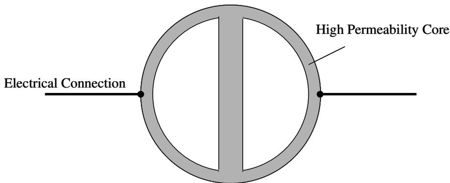
We now wind a toroidal coil around the ring core and feed it with DC so as to create a uniform field around the ring.
