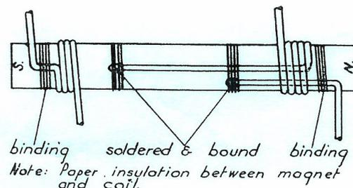
This winding diagram shows coils wound at each end, but the circuit diagram indicates a single coil wound over the length of each magnet.
