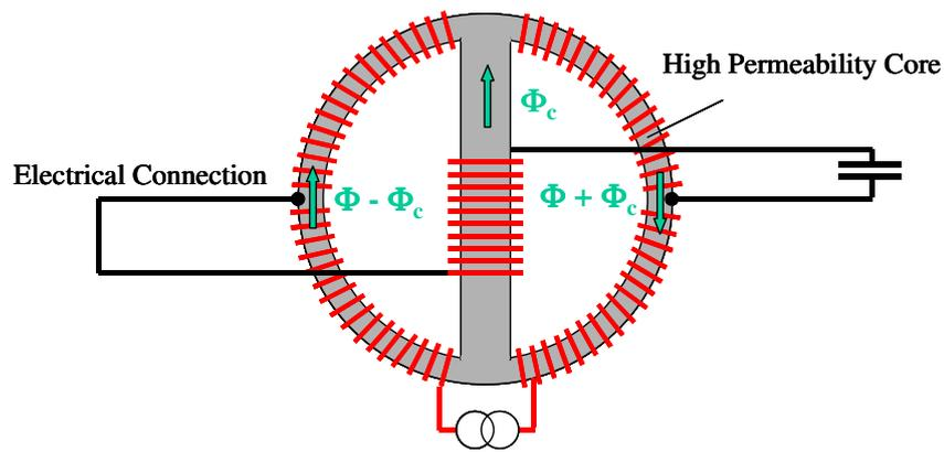
We now connect the center coil in series with a capacitor and in series with the core connections. Since the anomalous voltage across the core now depends on the resonant circuit current which flows through the core, the core will act like a resistor and if we get the polarities right it will be a negative resistor. If that value of negative resistance exceeds the positive resistance losses of the tuned circuit, it will self-oscillate.
