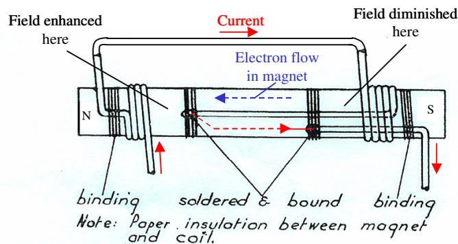
With the coil current alternating in direction, the field gradient will also alternate. Hence there will be an alternating voltage induced across that central region. The next image shows the alternate current flow where again the field gradient drag aids the flow.
