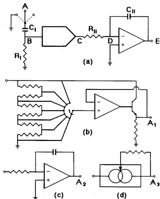
Fig. 1. (a) The multiplier-integrator circuit. (b) Variable voltage source. (c) Ramp generator for constant  $dV/dt$ . (d) LM334 current pump.
