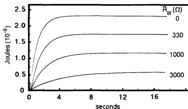
Fig. 3. Energy dissipated in  $R_1$  (1 k $\Omega$ ) vs time when  $C_1$  is charged from capacitor of equal capacitance through different resistors  $R_{III}$ .
