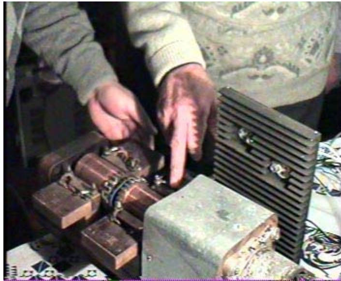
The mechanical commutator
