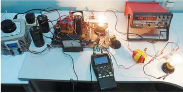
The photo clearly shows that both light bulbs are almost lit the same way. At the same time in the experiment: input power consumption DC 135 - 140 W (of which about 20 - 25%), and the net power on two lamps exceeds 200 watts. Total net power plus losses exceed 230 - 235 W at the entrance of 135-140 W
