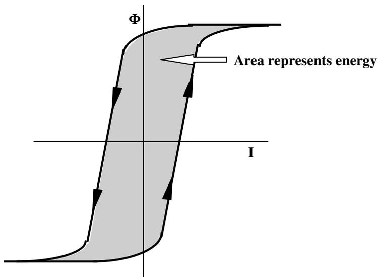
This  $\Phi$  v I plot is particularly useful when the flux passes through several materials having different magnetic characteristics.
