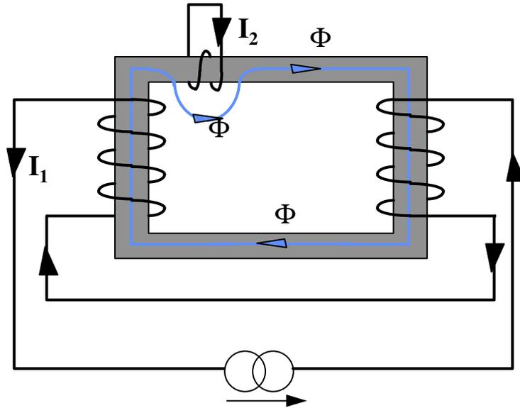
The flux is not excluded from the entire core, but mainly in the local region around the shorted coil, the induced current  $I_2$  creates the mmf necessary to force the flux through the air reluctance. We can move the shorted coil along the core with the same result.
