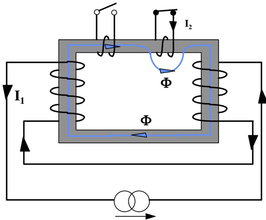
Then we can supply a short to the other before open circuiting the first coil, the flux exclusion zone simply jumps from one coil to the other.
