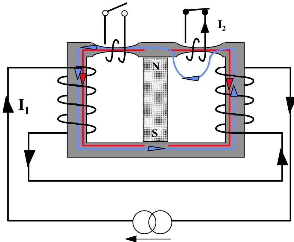
If we put a capacitor and load resistor across the exciter coils, the resonant circuit will be sustained by this output energy. We might also use some input energy to the switching coils to (a) get the system going and (b) make good the losses affecting the current induced into these coils.
