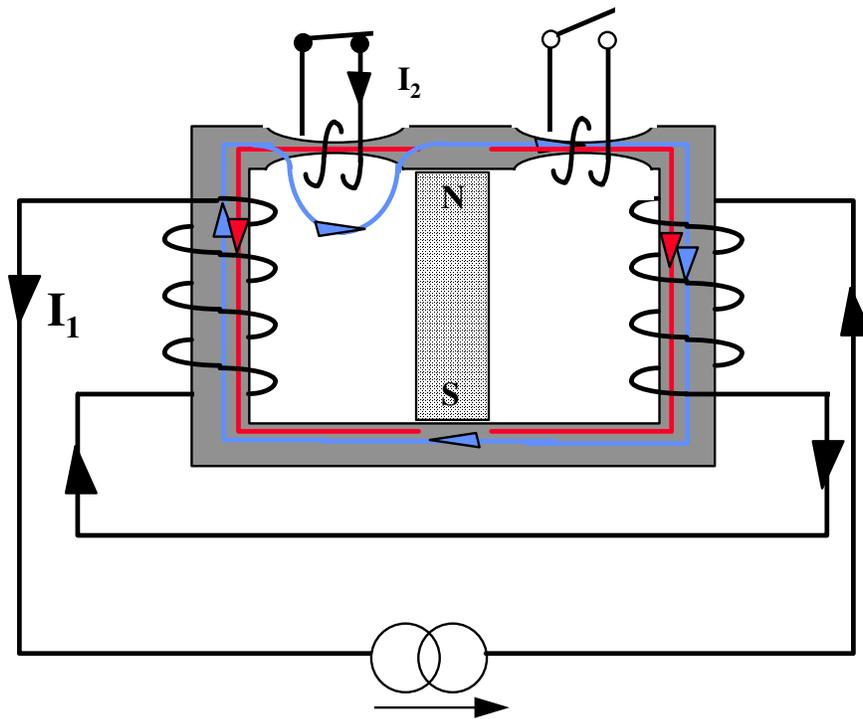
We arrange to short-circuit the left hand coil while, in the right hand region, exciter flux (blue) adds to magnet flux (red) so as to saturate. In this positive-going flux phase the left hand saturation region does not contribute because the flux change is excluded from it. We get one half of the synthesized characteristic
