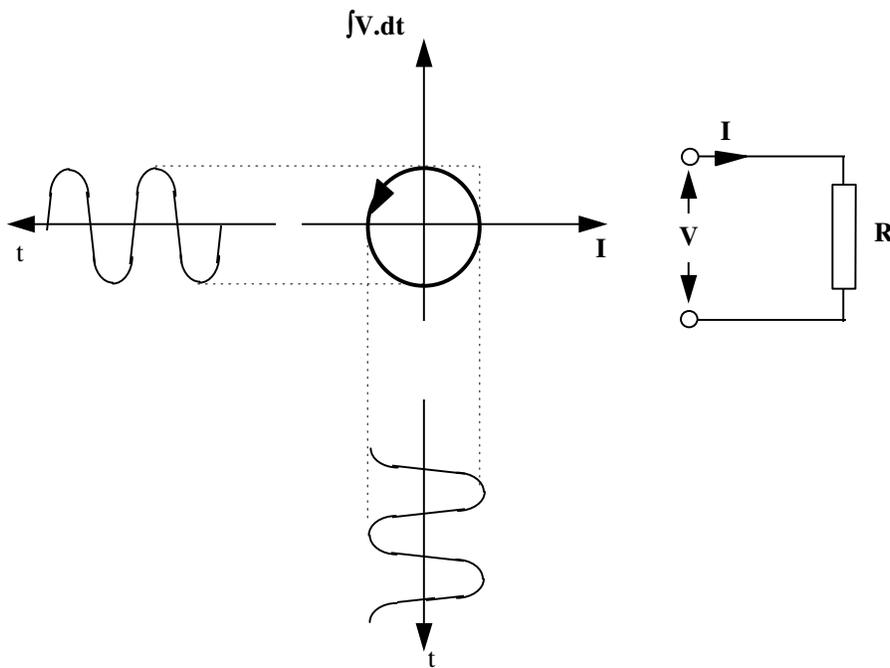
The plot forms a circle or ellipse whose area represents the energy lost as heat per cycle. Note the area is traversed anti-clockwise.
