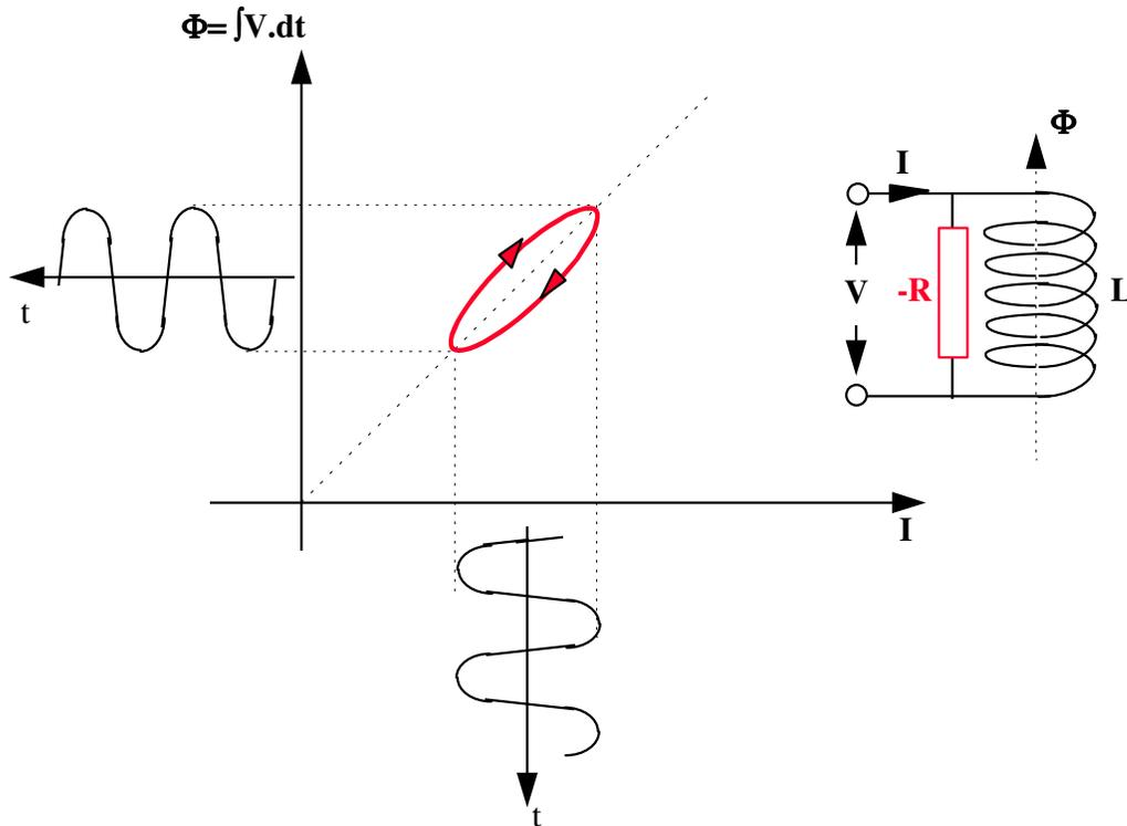
Note that now the area is traversed *clockwise*. It represents the energy per cycle flowing backwards from the  $-R$  source.
