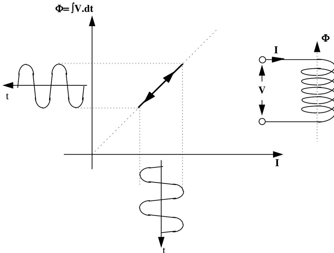
When driven by an AC source voltage and current are in phase quadrature, hence the voltage integral is in phase with the current. The  $\Phi$  v I plot yields a straight line whose slope is the inductance  $L$ .
