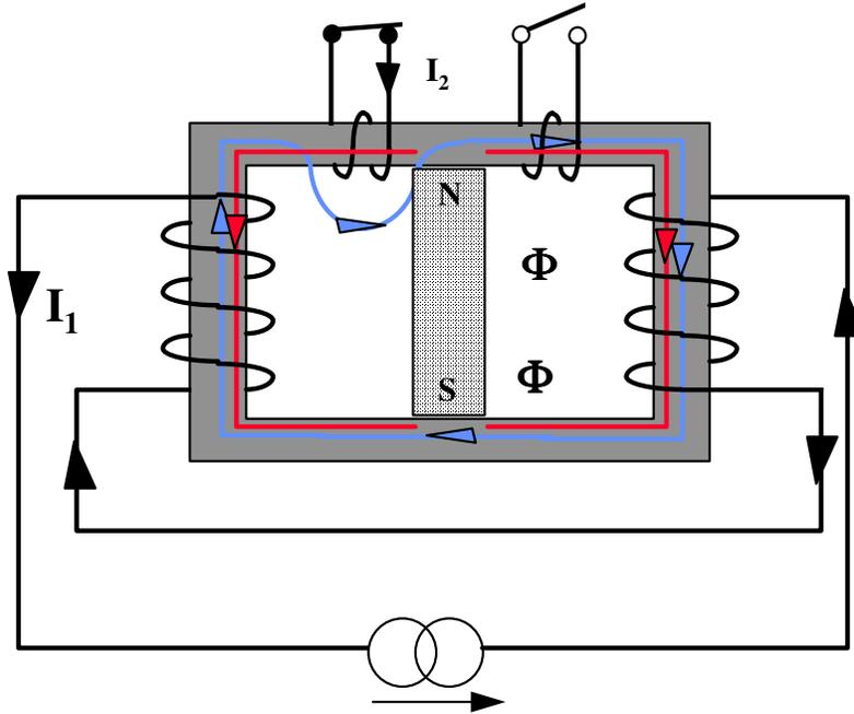
The magnet flux divides between the two core halves, and adds to the excited flux, but at this stage there is no OU, even when the core is driven to saturation.
