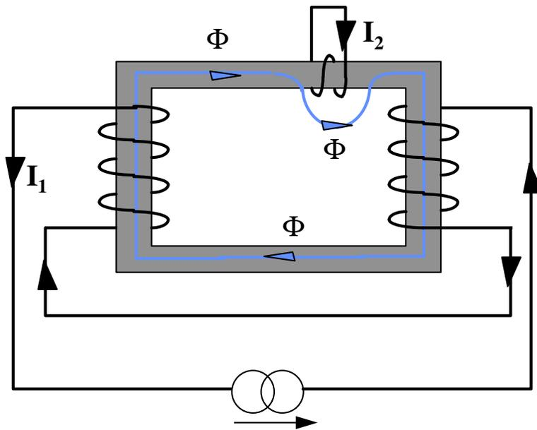
We can also have two switching coils, with flux initially forced out of one.
