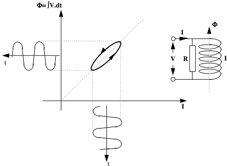
In the limit, when the resistor value is very small compared to the reactance of the inductor, the flux disappears but the voltage integral remains. We get the following figure.
