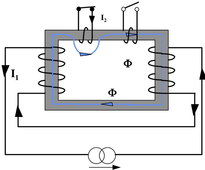
*Note the flux through the two main exciter coils remains the same, the switching action is not “seen” by the current source  $I_1$ .*
