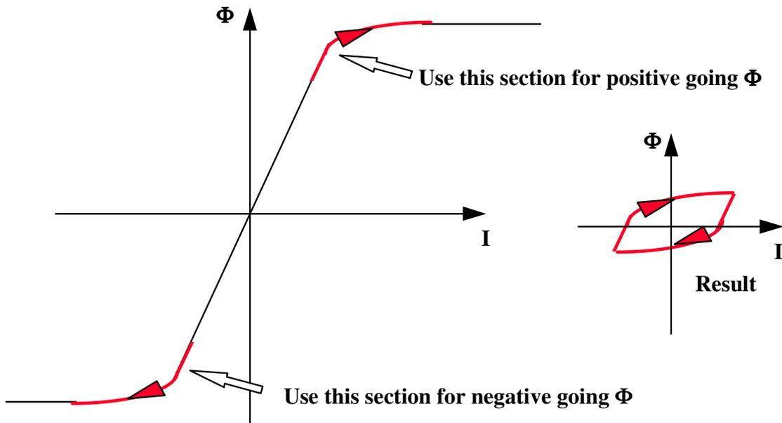
If we could arrange for flux within a coil to be positive-going while also going over the positive saturation knee, then when negative-going it does not trace its original steps, but passes over the negative saturation knee, we would get the combined characteristic we desire. The following section is devoted to this possibility.
