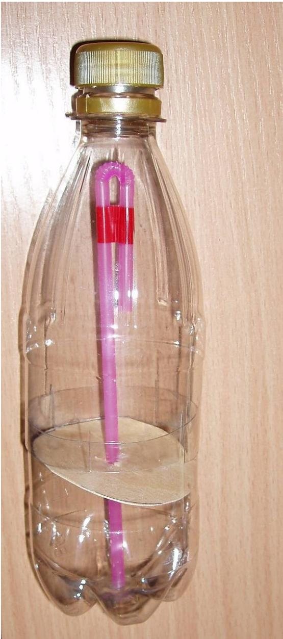
put upper part of the bottle on the bottom so that they overlap about 1cm (so that two “petals” of the top bottle part between incisions go inside bottom part and two “petals” left outside)
