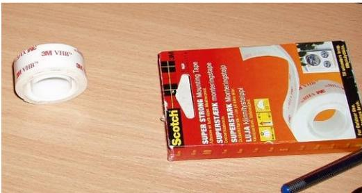
use dual side adhesive mounting tape to temporary fix porous membrane if necessary
