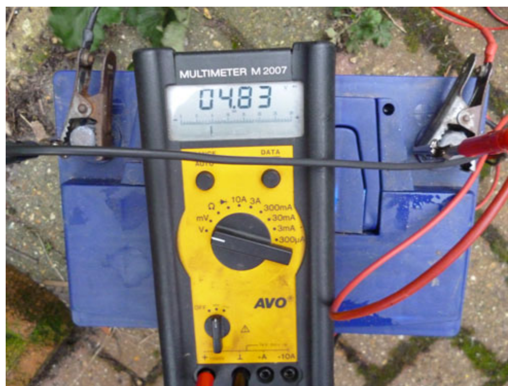
this battery was discharged to 4.83V open circuit, way too low below 11.5V
