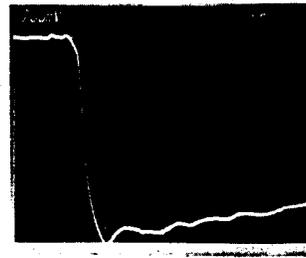
FIG. 3. Output of MOSFET pulser. 200 V/div and 5 ns/div.
