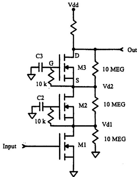
FIG. 1. Reliable method of stacking power MOSFETs.
