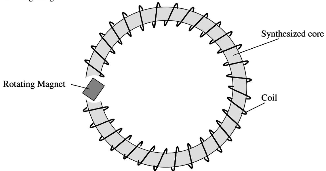
The inductance of such a coil where the air gap is small compared to the length of the coil is given closely by
