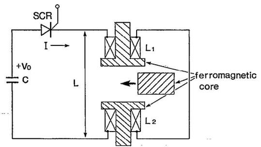
FIG. 3. LCR circuit with two coils and a movable ferromagnetic core inserted between the coils.
