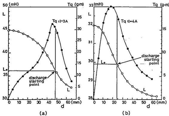
FIG. 6. Combined inductance ( $L$ ) and torque ( $Tq$ ) between the electromagnet and the ferromagnetic core. The torque was measured under conditions of constant current. Values of  $L$  and  $Tq$  for (a) the attracting mode, and (b) the opposing mode.
