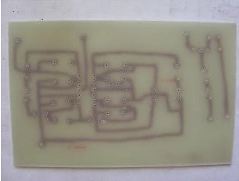
010.jpg is the top view of the printed circuit board for the swagatam ghost detector circuit.
