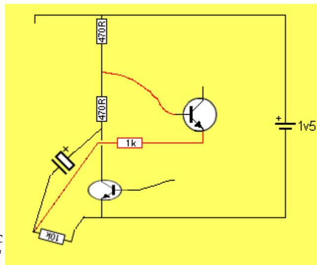
Next, we have the astable multivibrator, or FLIP FLOP [pronounced (h)ay stable] - meaning it has unstable states. In this case, two unstable states.
