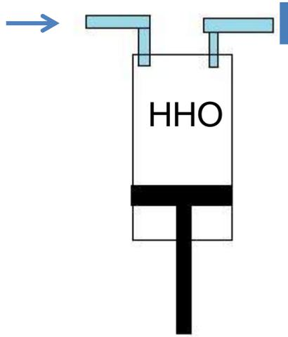
1. HHO gas goes into combustion chamber at atmospheric pressure.
