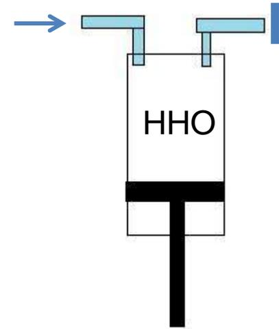
3. HHO gas goes into Combustion chamber at slightly higher than Atm Pressure. Or Weight of Piston in Diagram helps.
