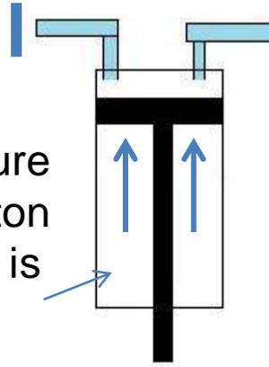
2. HHO gas ignited. Partial vacuum created. Atm Pressure pushes Piston upwards. Work done by External Atm Pressure. Exhaust valve can remain shut! Practically no exhaust gas!
