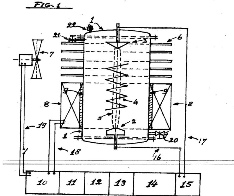
Figure 1 shows the v.n.l. heat-producing reactor, as well as the electric circuit.
