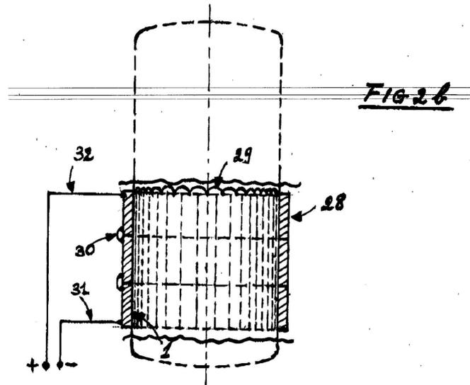
and Figure 2b shows implementation with bi-metal-> electret stacks, to the reactor outer wall. Figure 2b: Infra-red photo volts. cells (eg, 12 cm x 3 cm, each) at the entire periphery of the exterior of the reactor (1), which comprise for example Ga / Sb (28); parallel compounds, (29); in-series compounds, (30); - Wire, (31); + Wire (32), both to charge battery (10).
