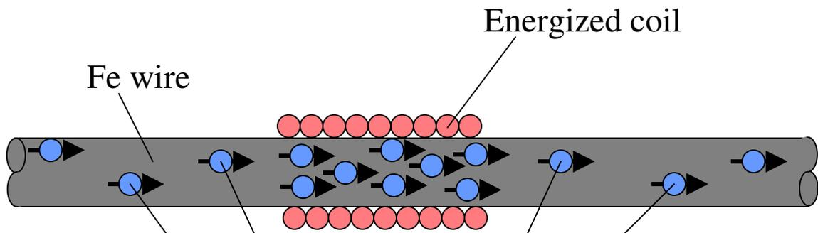
Conduction electrons are spin aligned with the magnetic field and get attracted by the magnetic gradient into the coil region.
