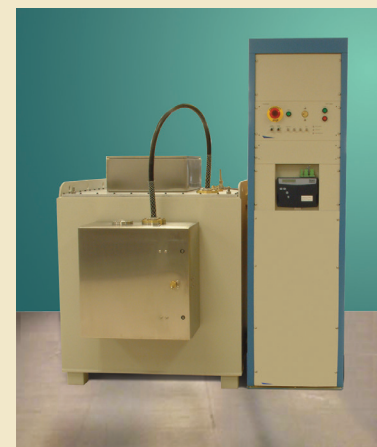
PEF treatment system for wastewater treatment (pre-digestion). This system is rated at 150 kW average power, and produces pulses up to 40 kV, 500 A. It processes 10,000 liters/hour of wastewater sludge prior to anaerobic digestion.
