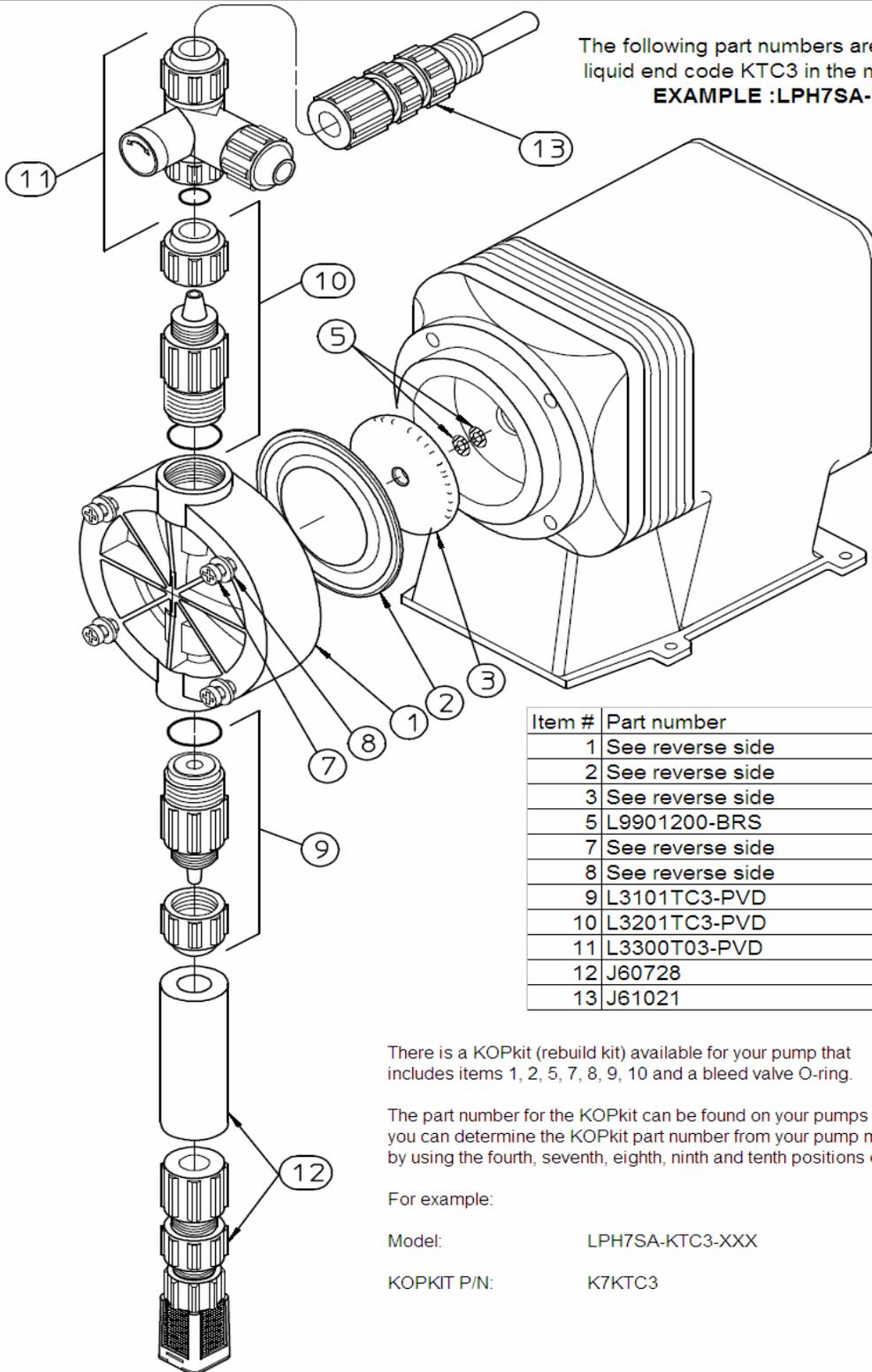
The following part numbers are for pump models with liquid end code KTC3 in the model.
