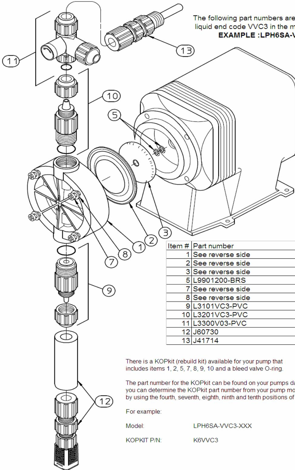
The following part numbers are for pump models with liquid end code VVC3 in the model.
