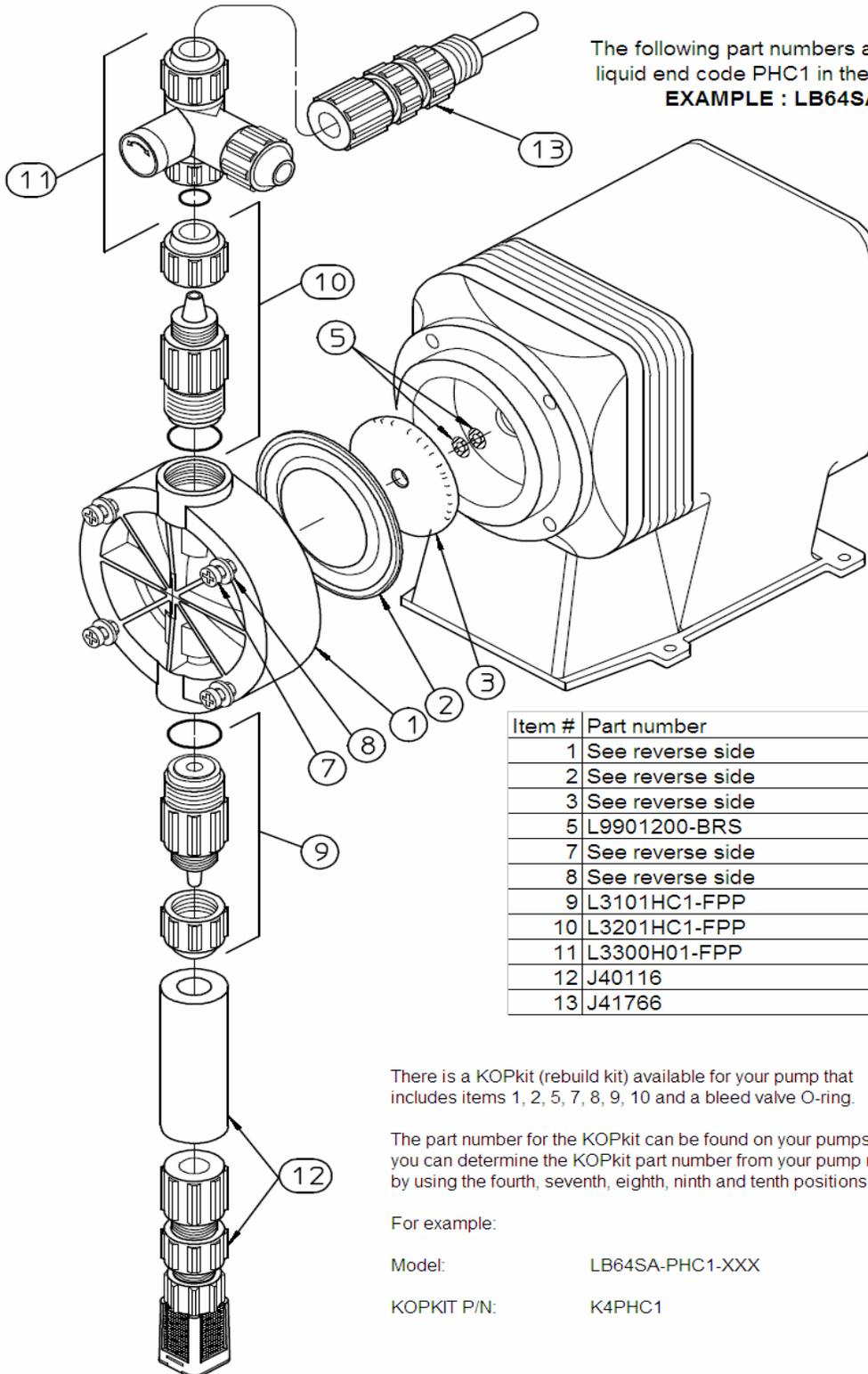
The following part numbers are for pump models with liquid end code PHC1 in the model.
