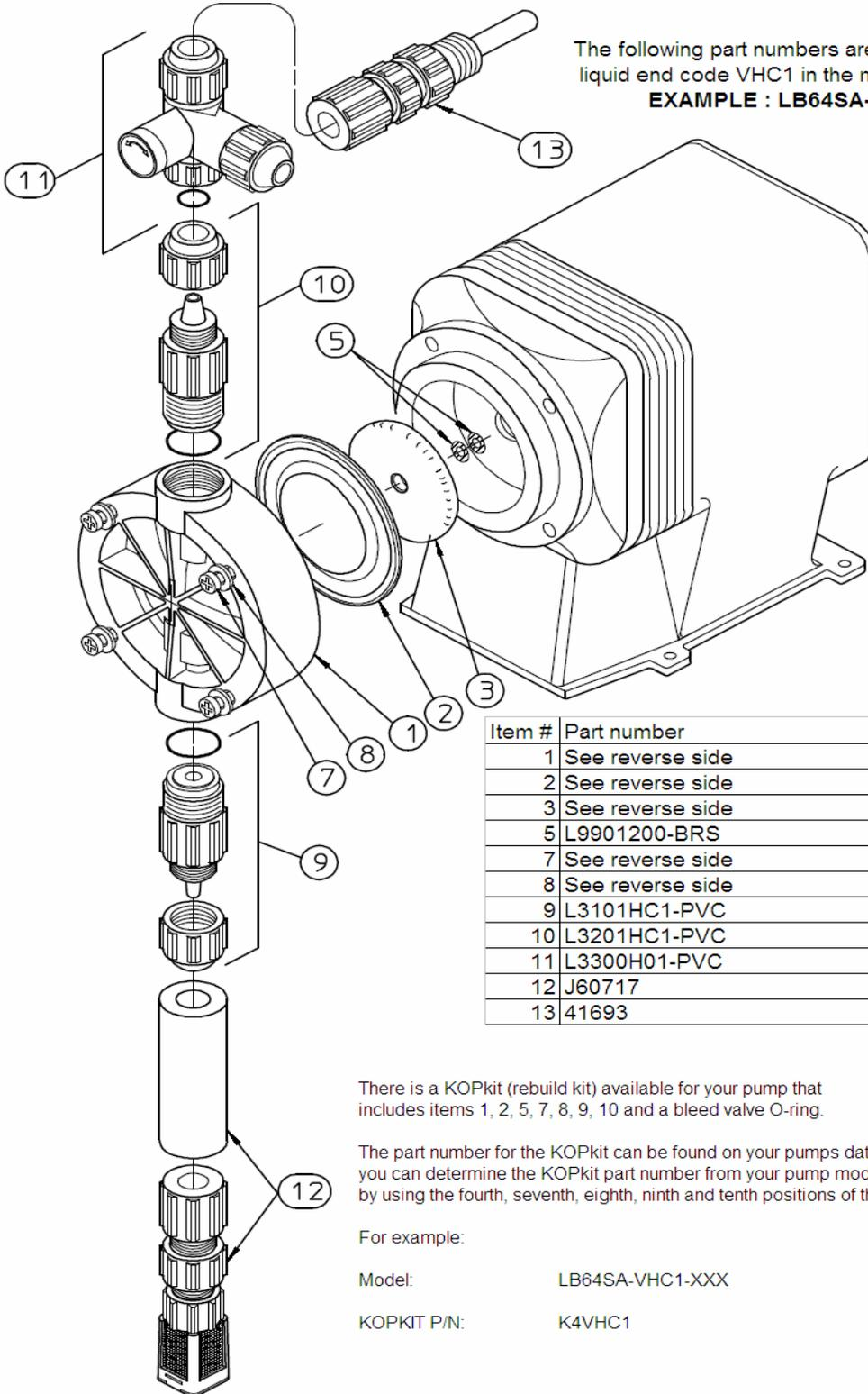
The following part numbers are for pump models with liquid end code VHC1 in the model.
