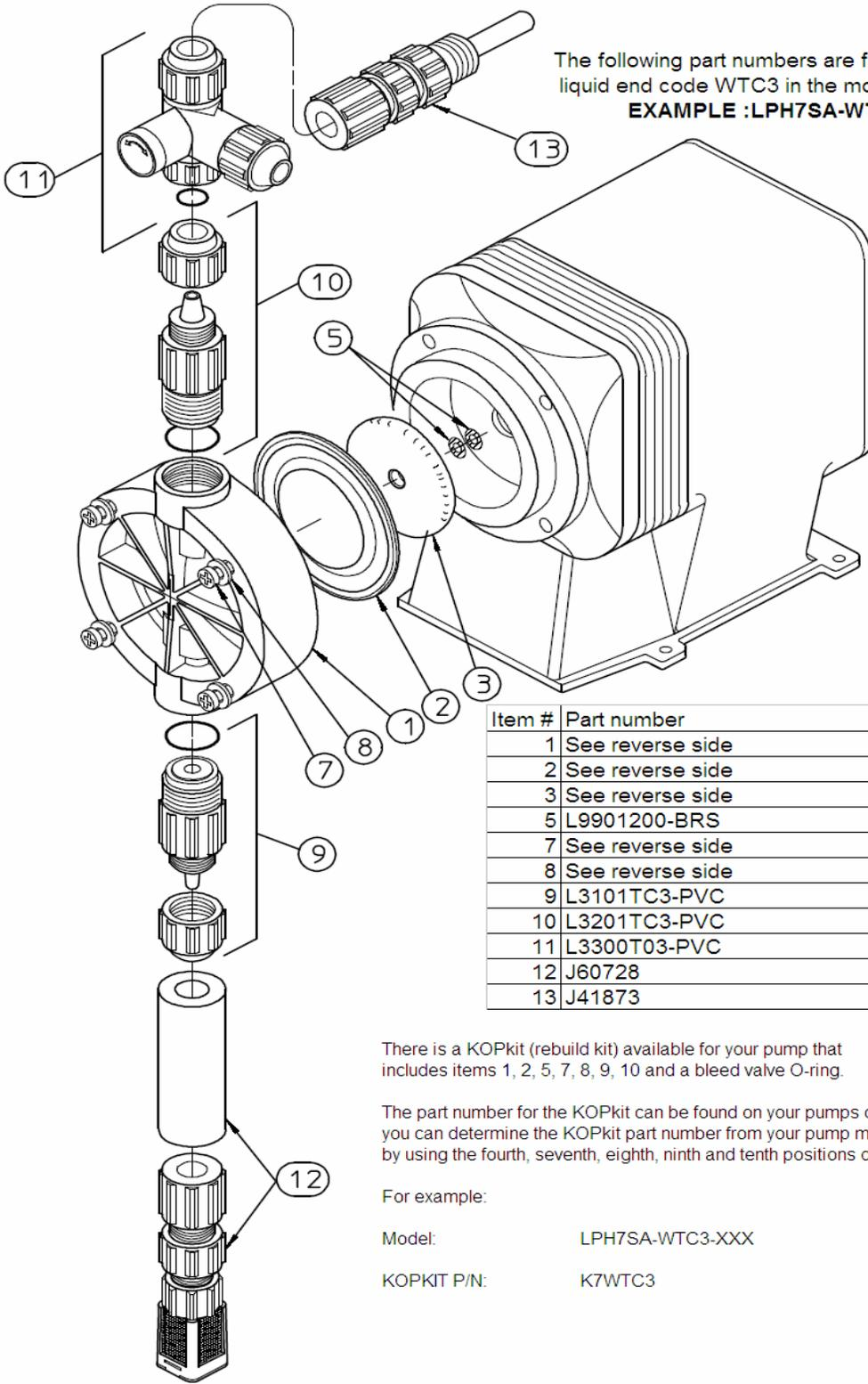
The following part numbers are for pump models with liquid end code WTC3 in the model.
