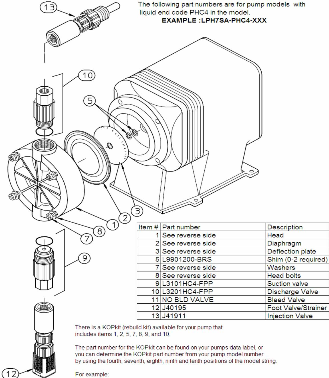
The following part numbers are for pump models with liquid end code PHC4 in the model.
