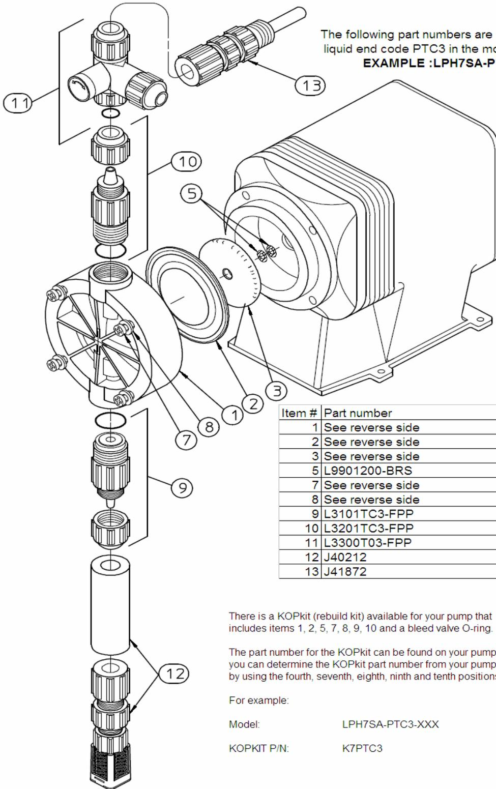
The following part numbers are for pump models with liquid end code PTC3 in the model.
