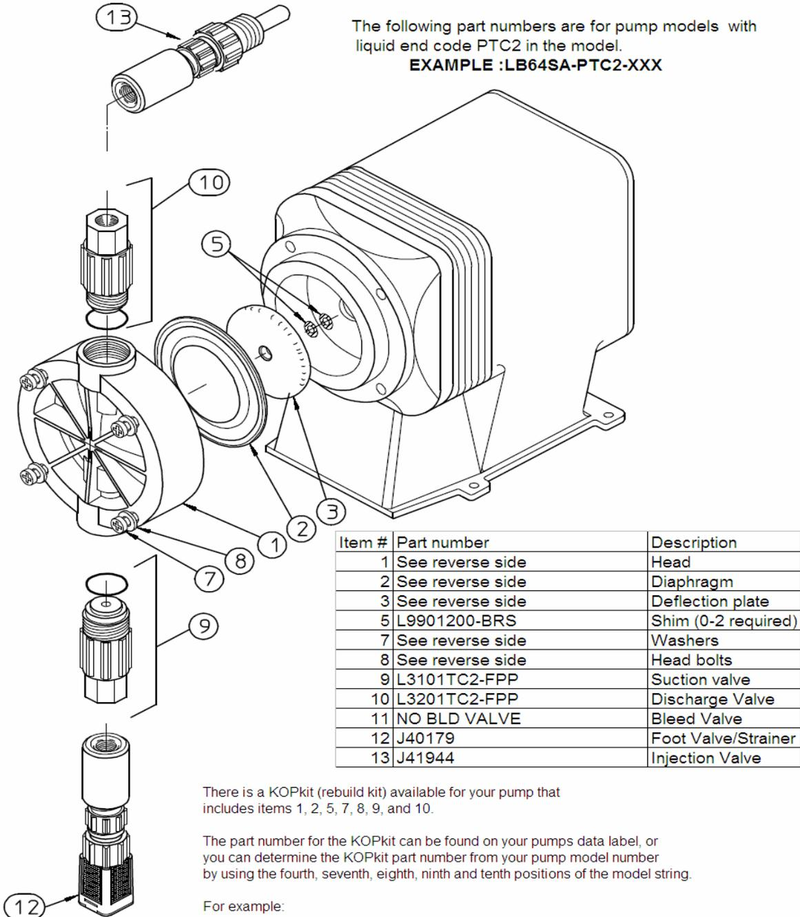
The following part numbers are for pump models with liquid end code PTC2 in the model.
