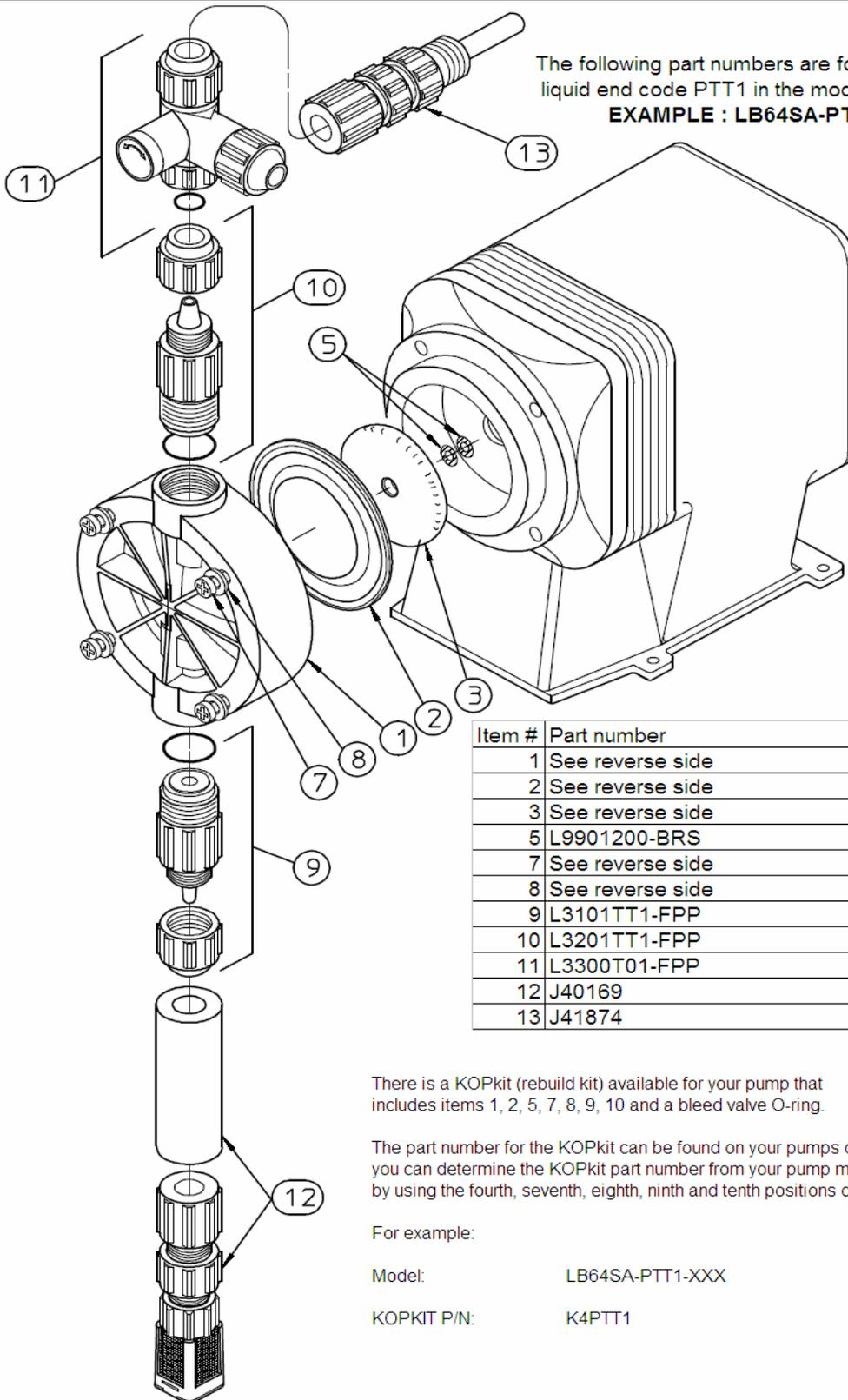
The following part numbers are for pump models with liquid end code PTT1 in the model.
