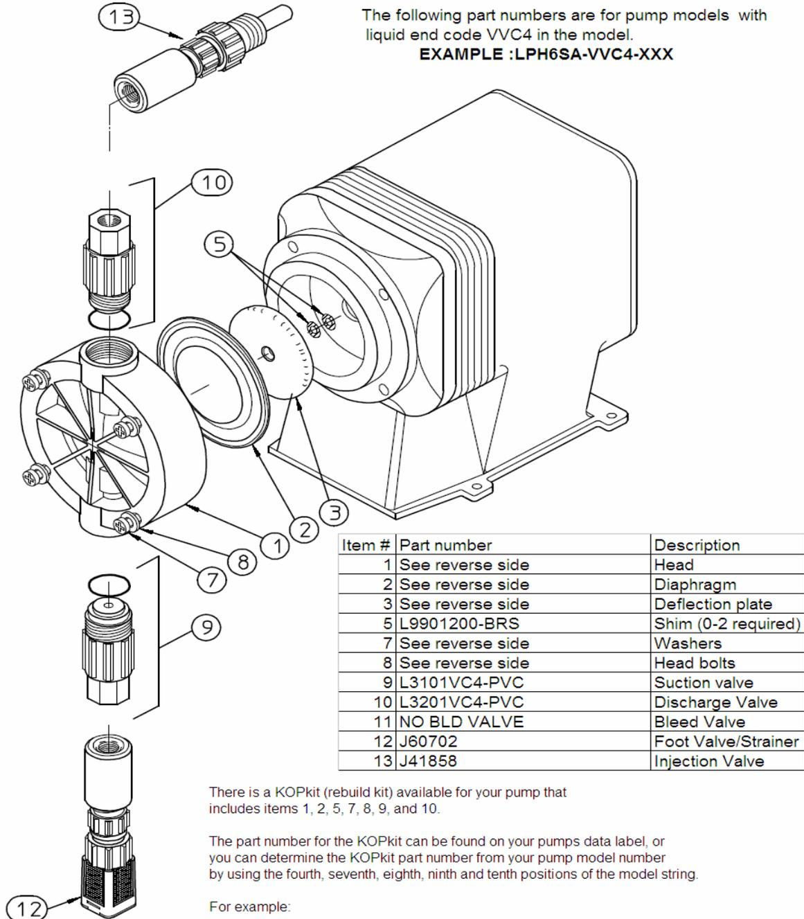
The following part numbers are for pump models with liquid end code VVC4 in the model.
