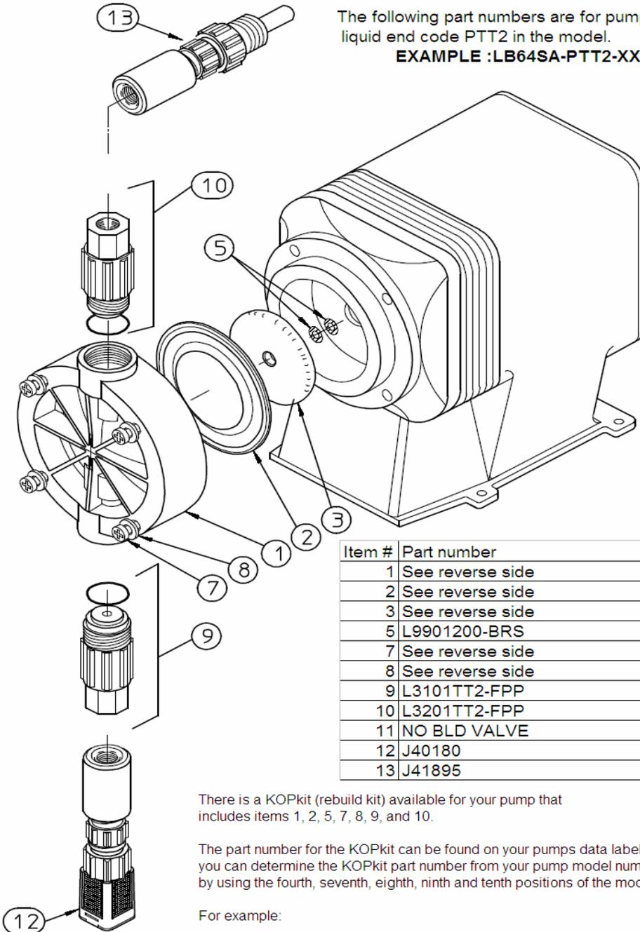
The following part numbers are for pump models with liquid end code PTT2 in the model.
