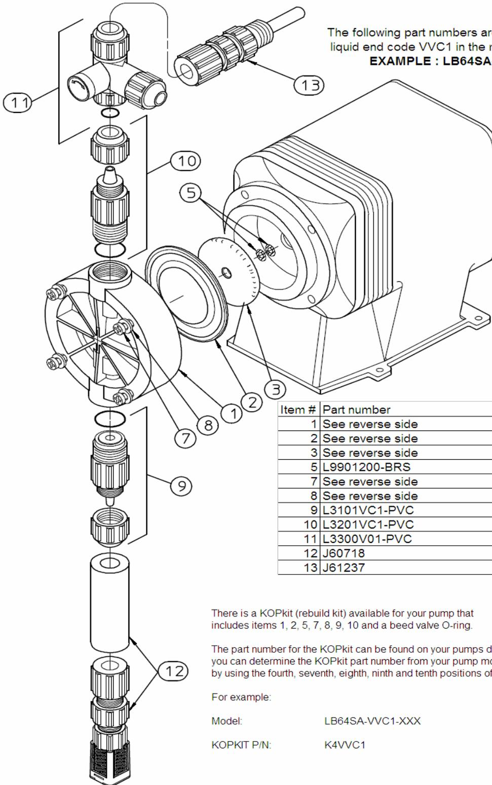
The following part numbers are for pump models with liquid end code VVC1 in the model.
