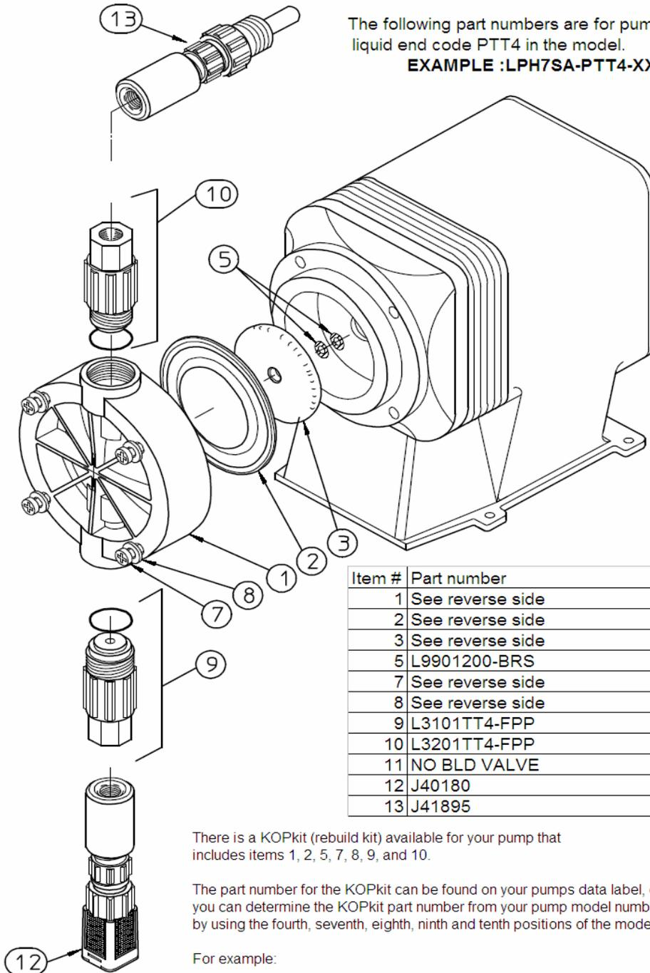
The following part numbers are for pump models with liquid end code PTT4 in the model.
