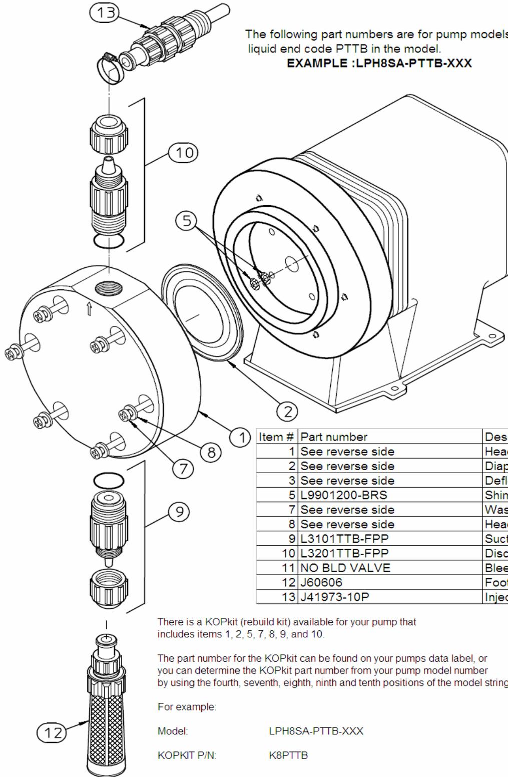
The following part numbers are for pump models with liquid end code PTTB in the model.
