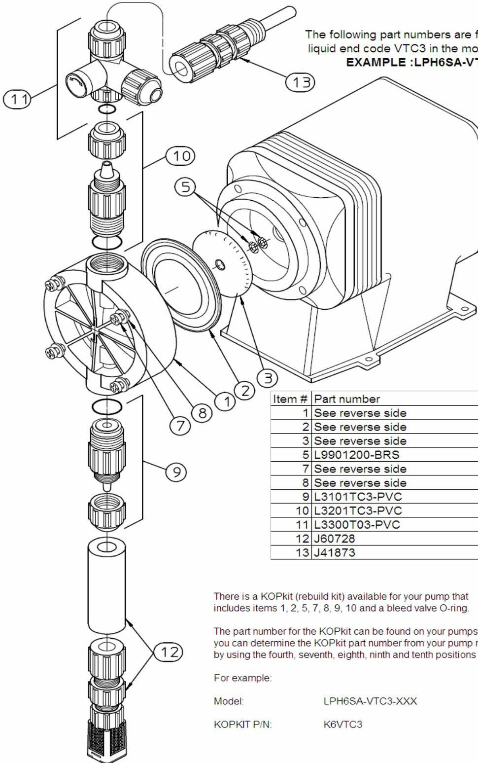
The following part numbers are for pump models with liquid end code VTC3 in the model.
