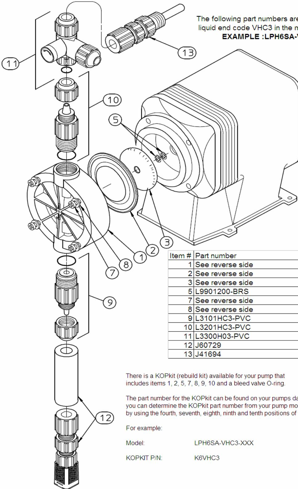
The following part numbers are for pump models with liquid end code VHC3 in the model.
