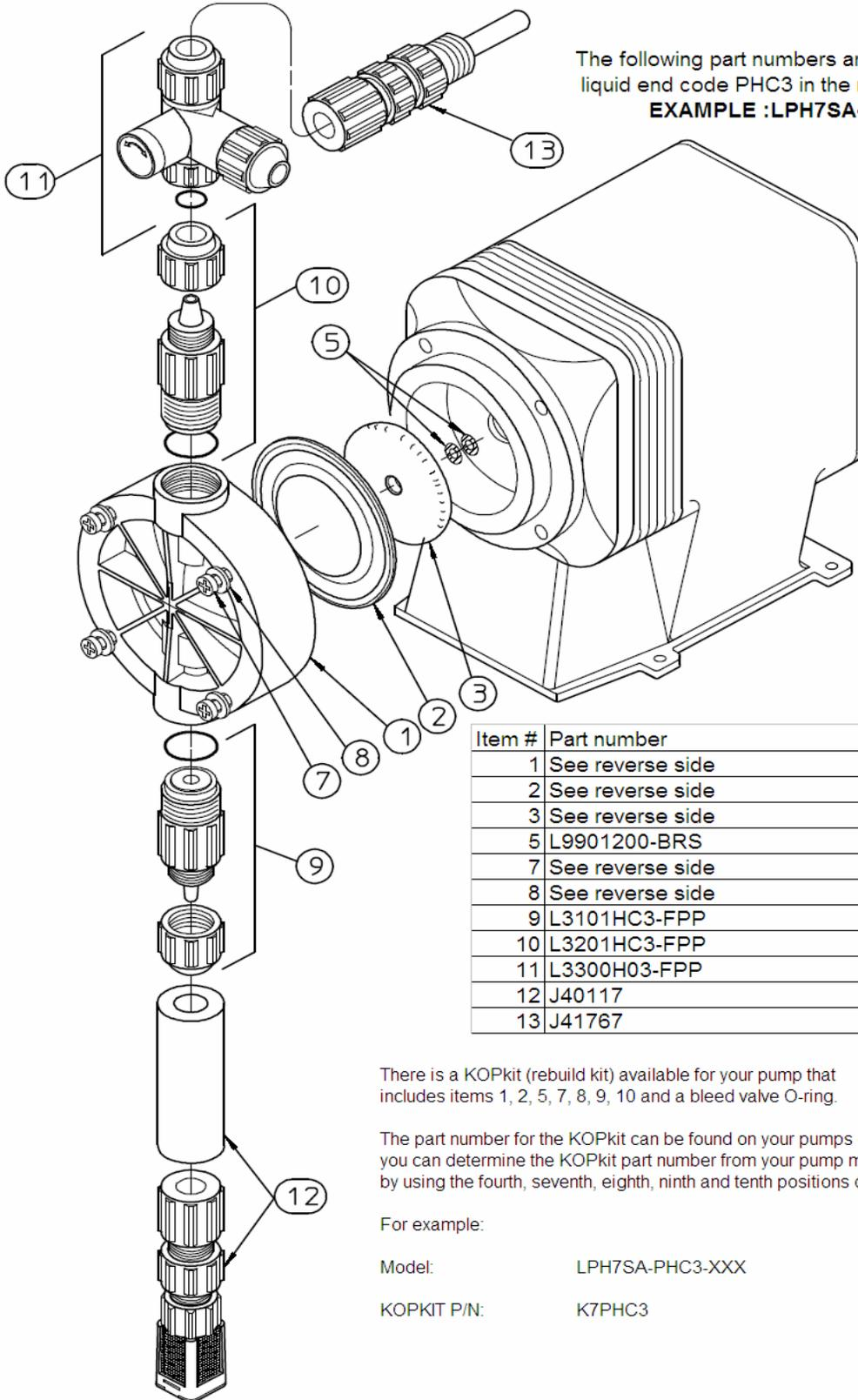
The following part numbers are for pump models with liquid end code PHC3 in the model.
