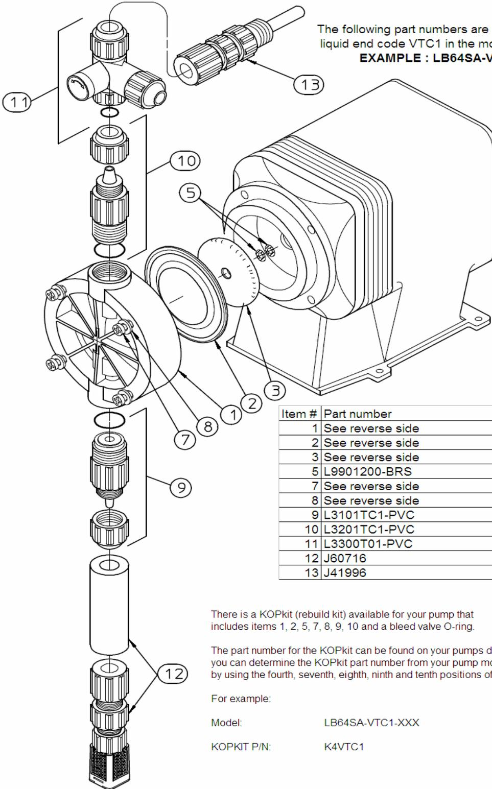
The following part numbers are for pump models with liquid end code VTC1 in the model.
