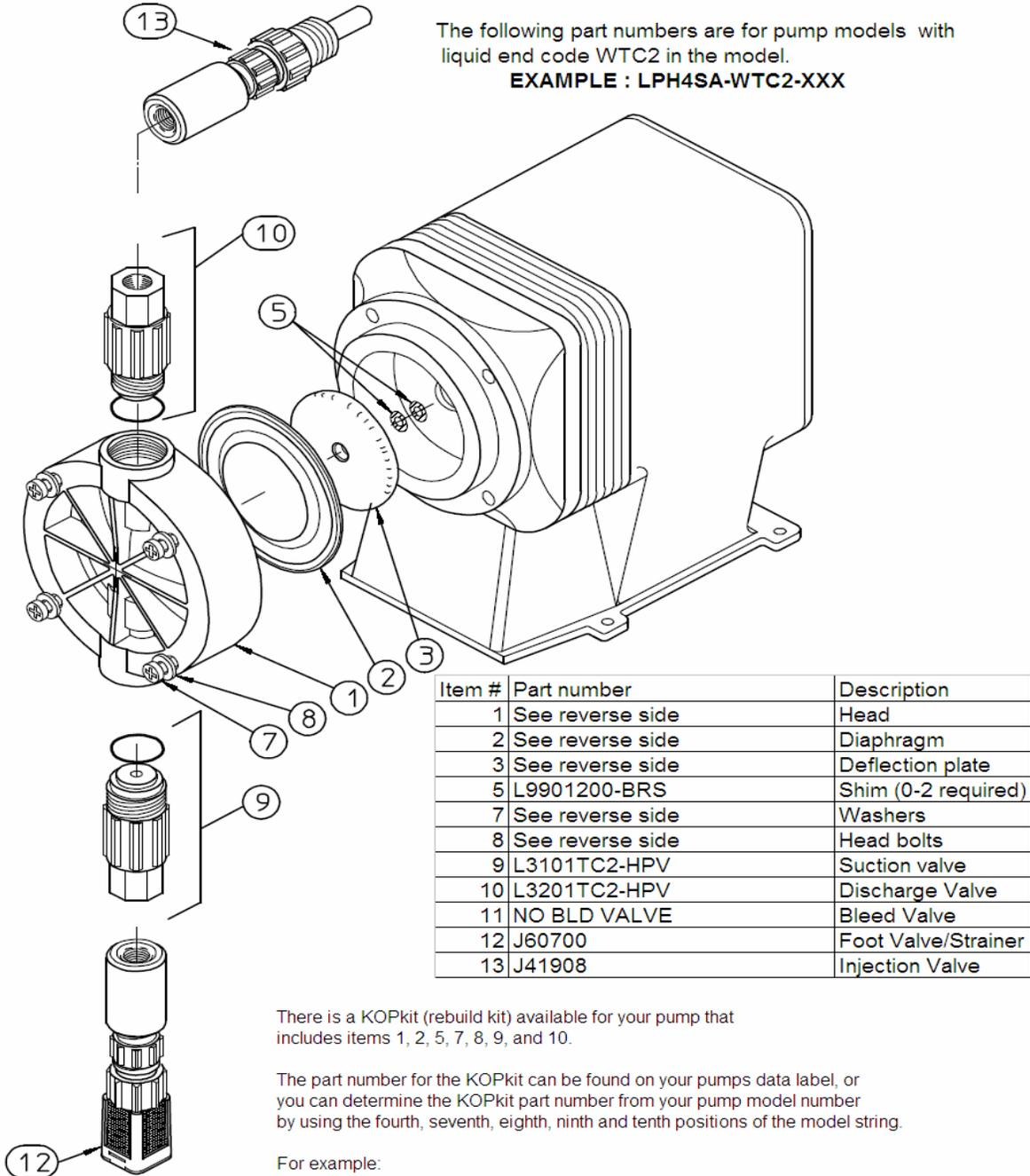
The following part numbers are for pump models with liquid end code WTC2 in the model.
