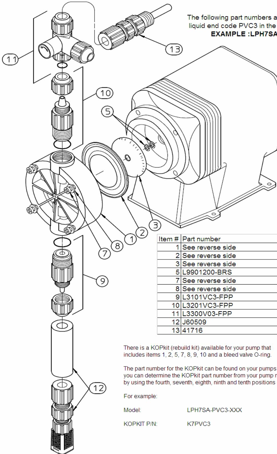
The following part numbers are for pump models with liquid end code PVC3 in the model.
