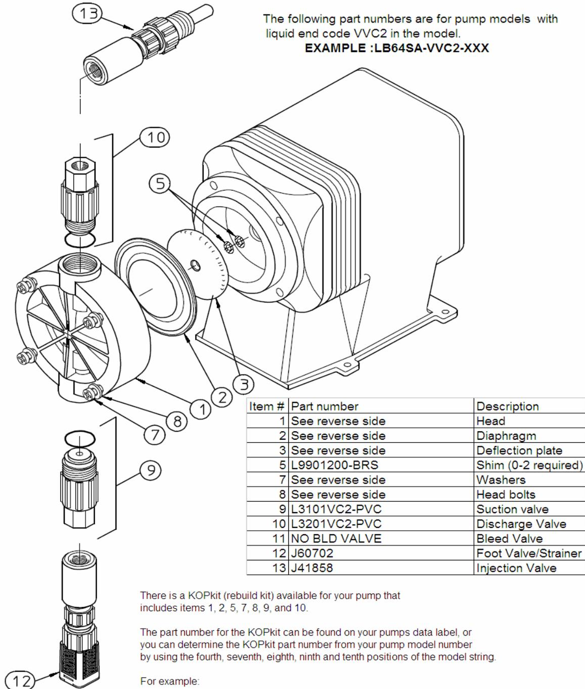
The following part numbers are for pump models with liquid end code VVC2 in the model.
