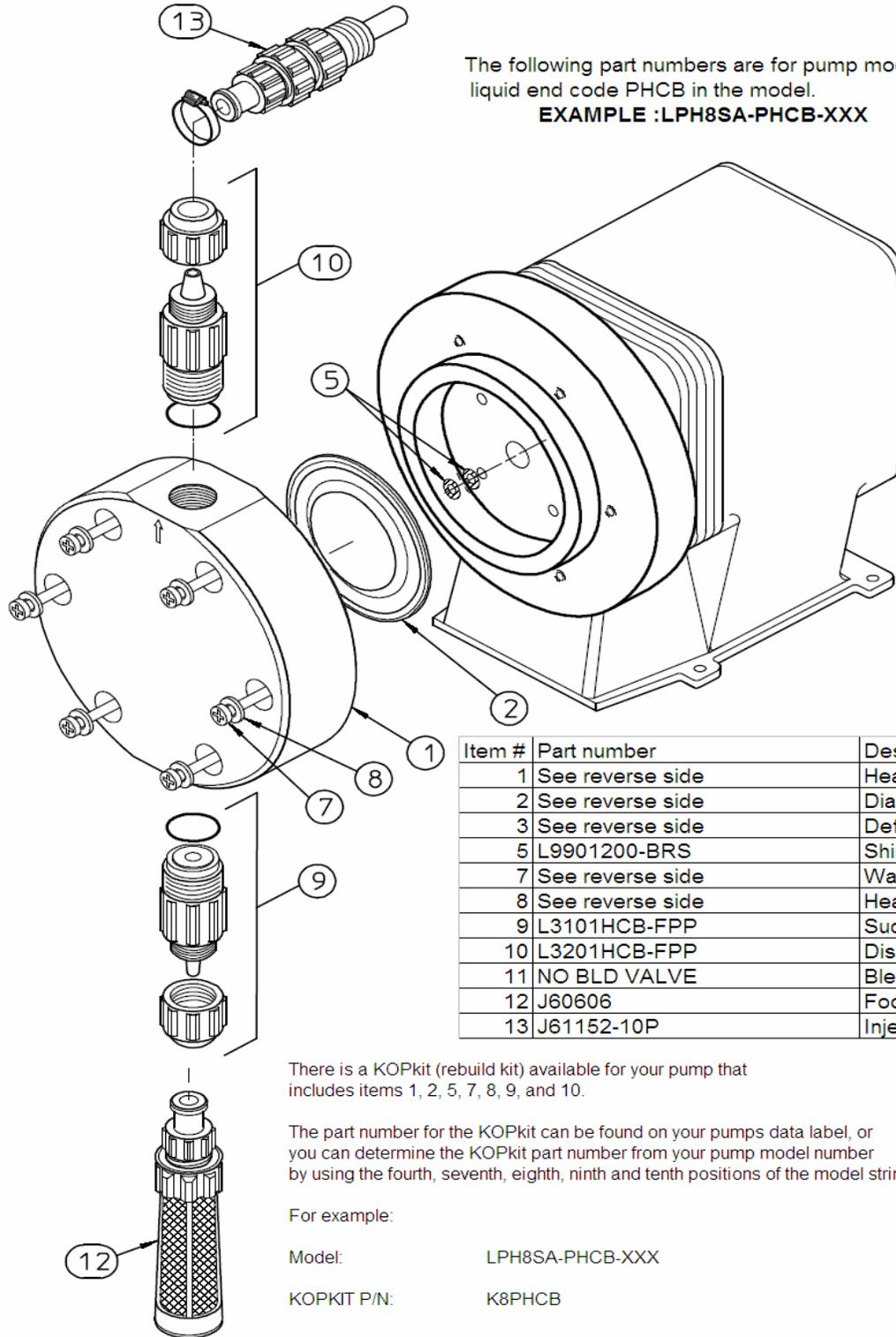
The following part numbers are for pump models with liquid end code PHCB in the model.
