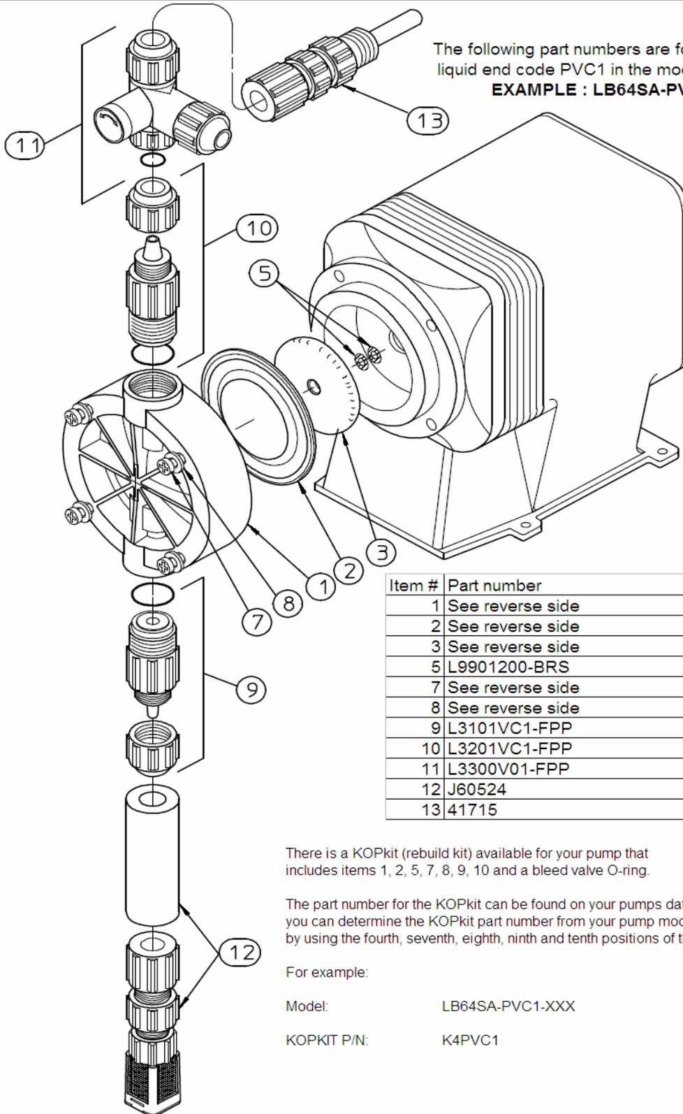
The following part numbers are for pump models with liquid end code PVC1 in the model.
