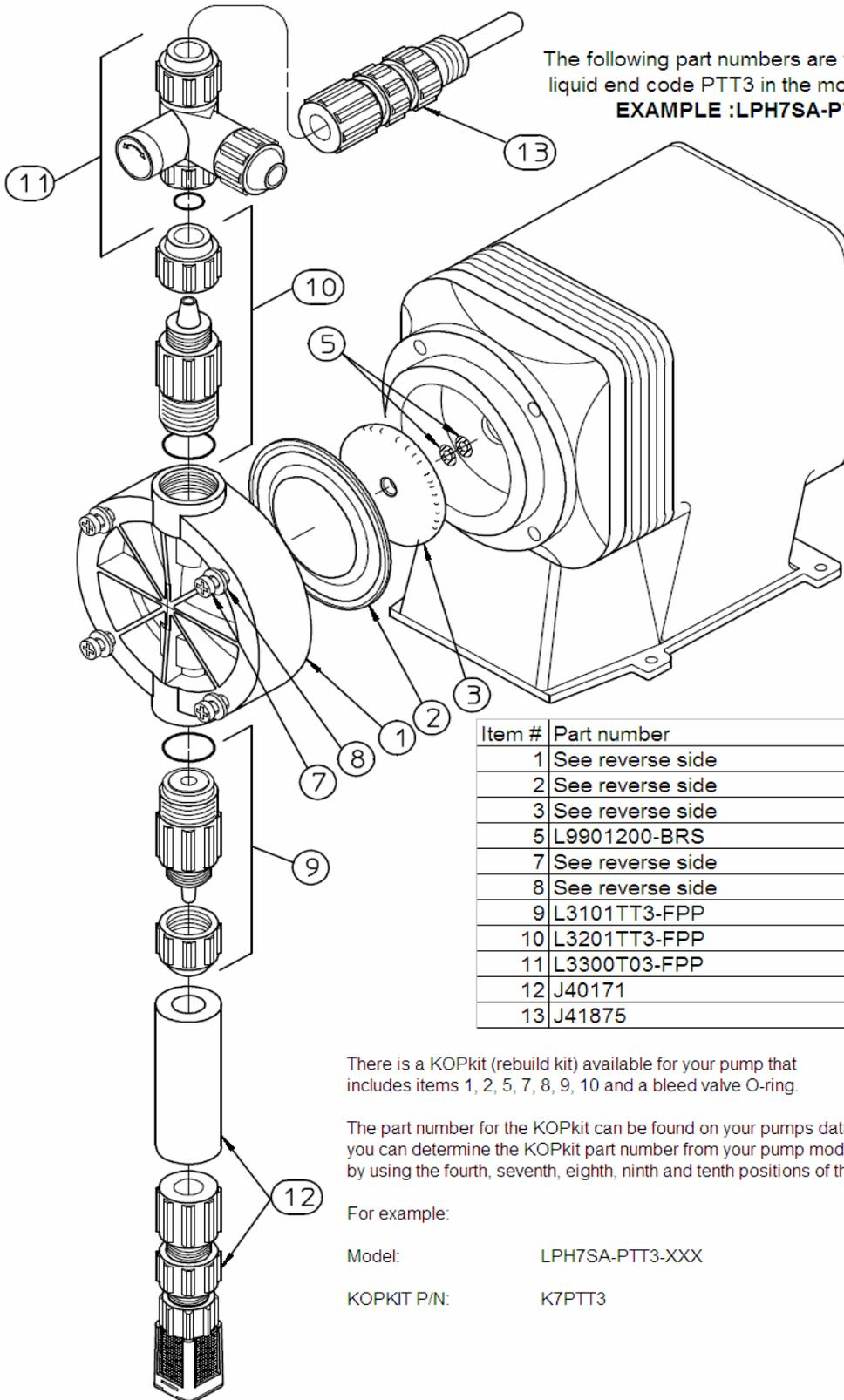
The following part numbers are for pump models with liquid end code PTT3 in the model.
