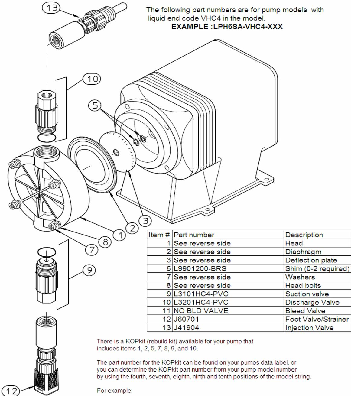
The following part numbers are for pump models with liquid end code VHC4 in the model.
