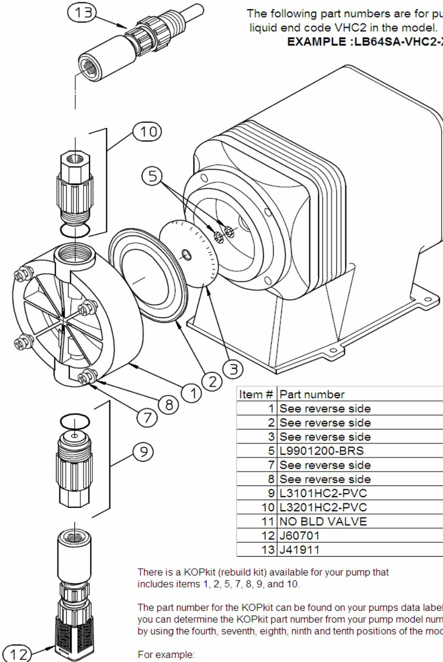
The following part numbers are for pump models with liquid end code VHC2 in the model.
