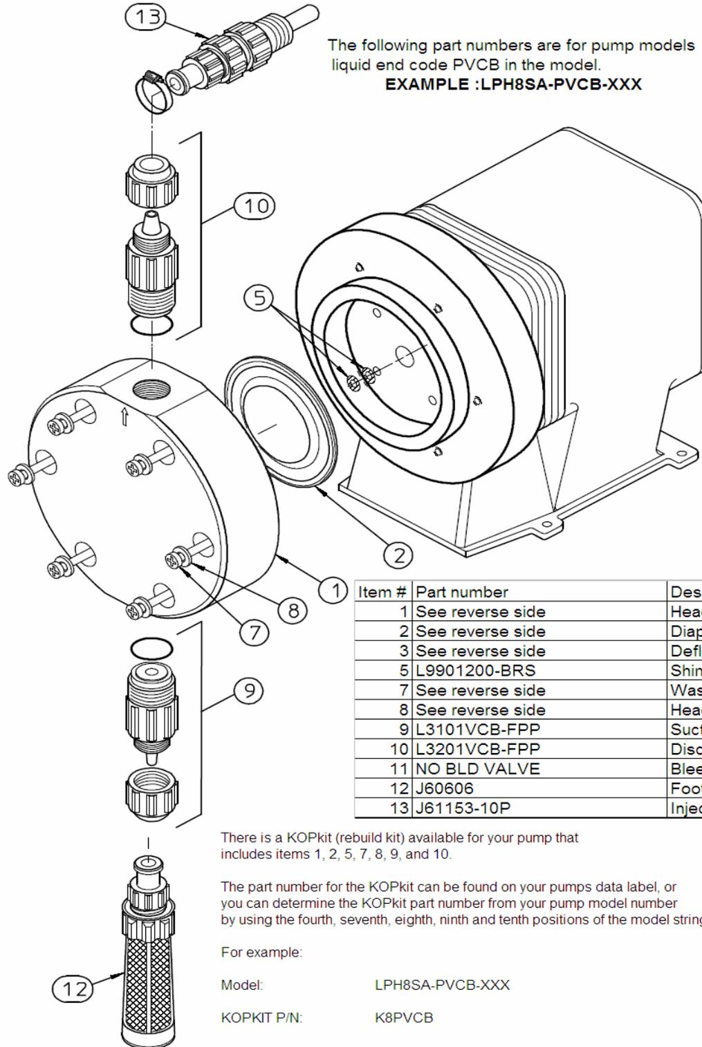
The following part numbers are for pump models with liquid end code PVCB in the model.
