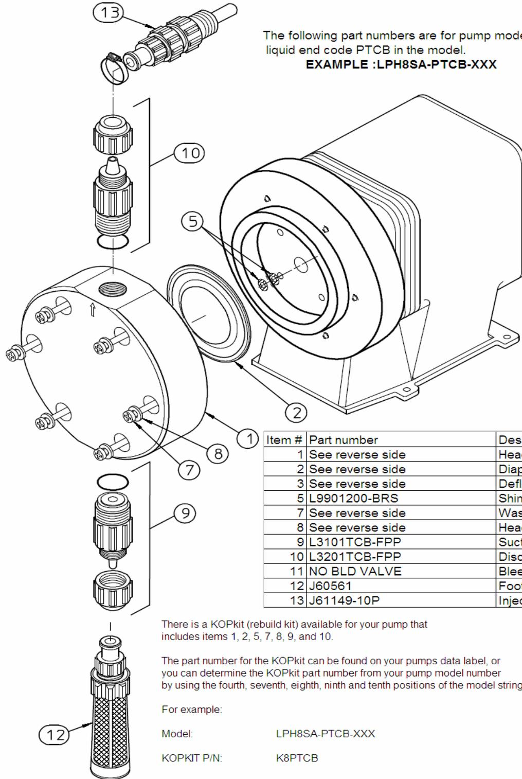
The following part numbers are for pump models with liquid end code PTCB in the model.
