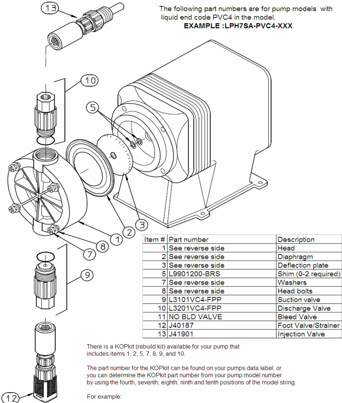
The following part numbers are for pump models with liquid end code PVC4 in the model.
