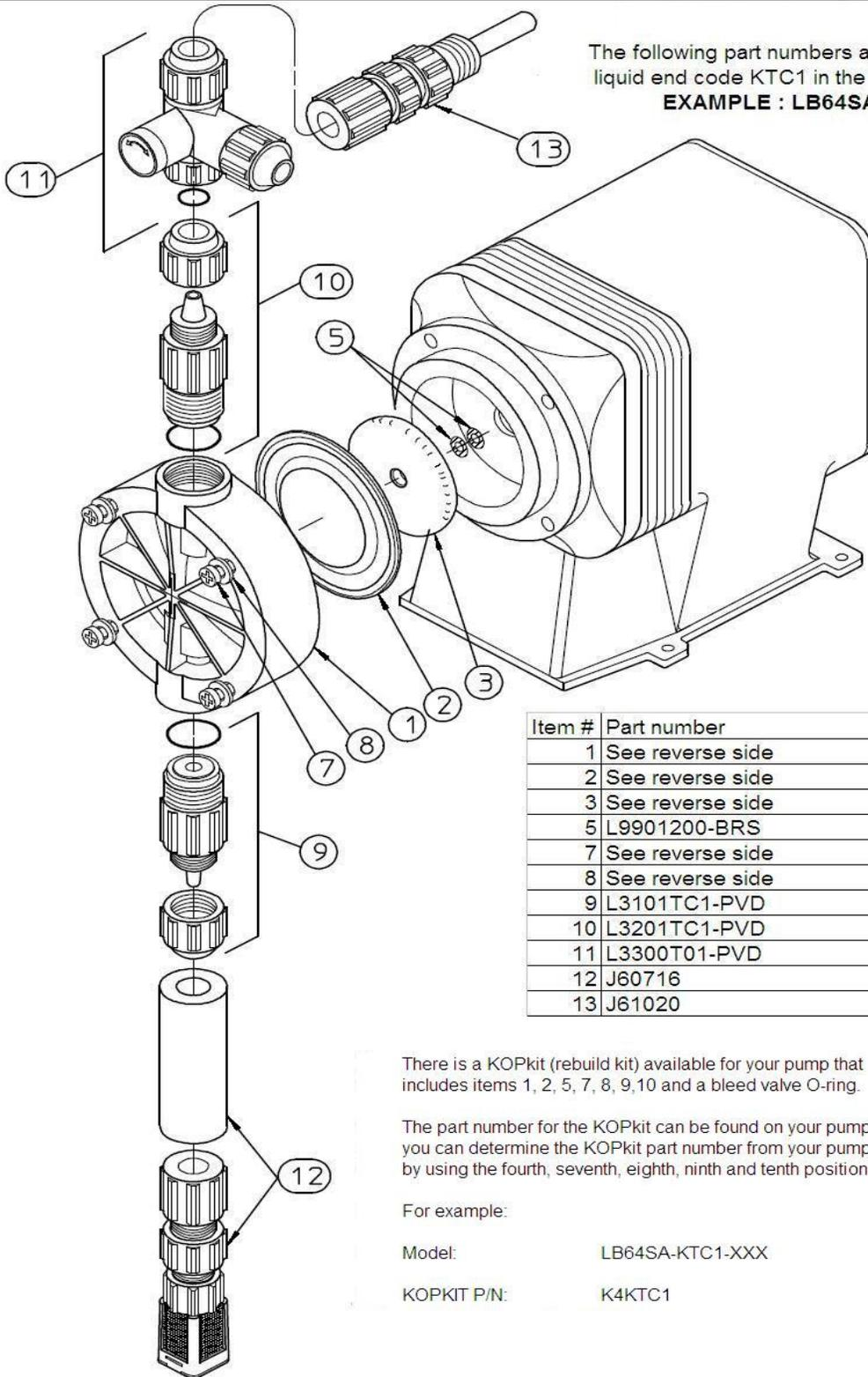
The following part numbers are for pump models with liquid end code KTC1 in the model.
