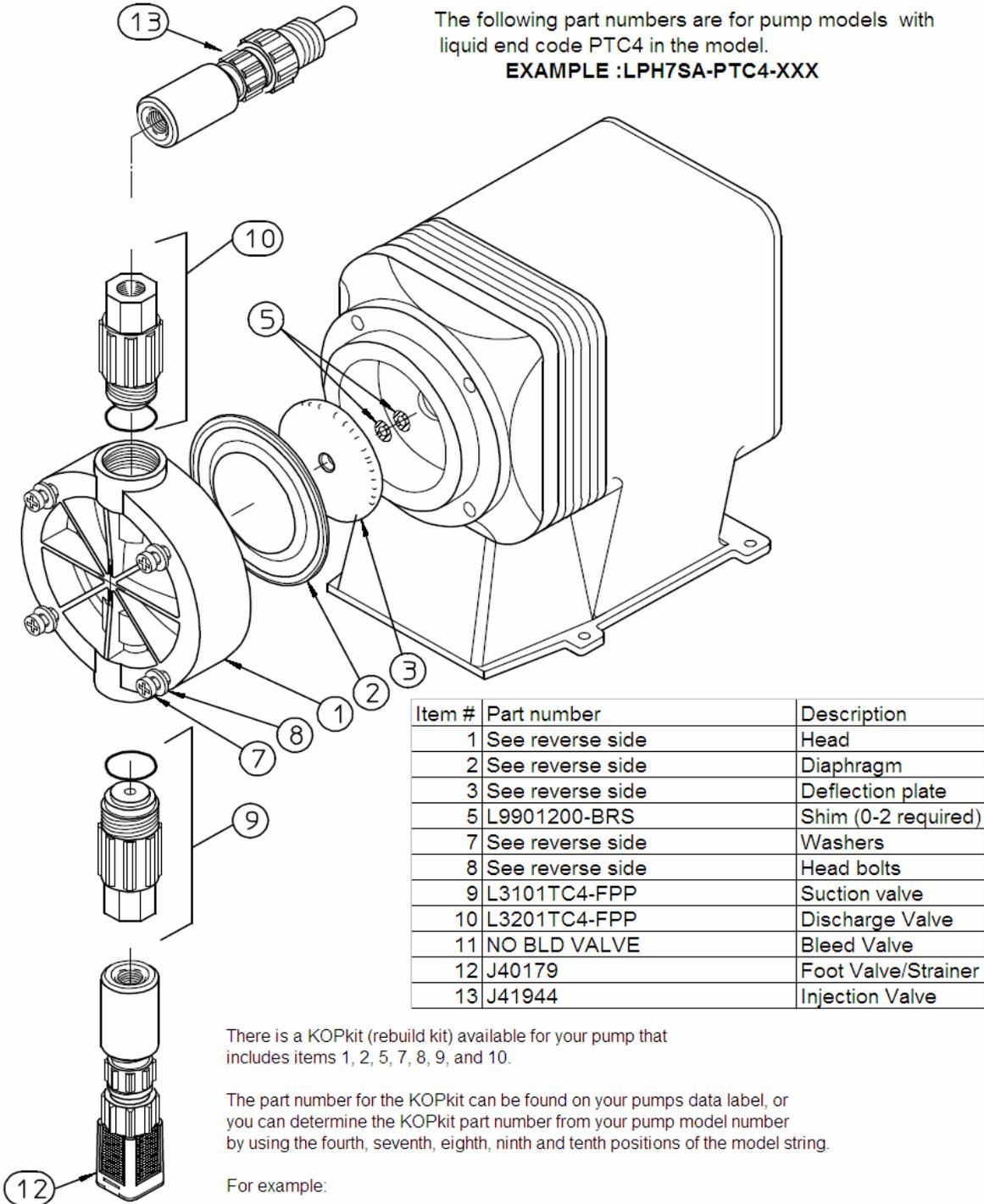
The following part numbers are for pump models with liquid end code PTC4 in the model.
