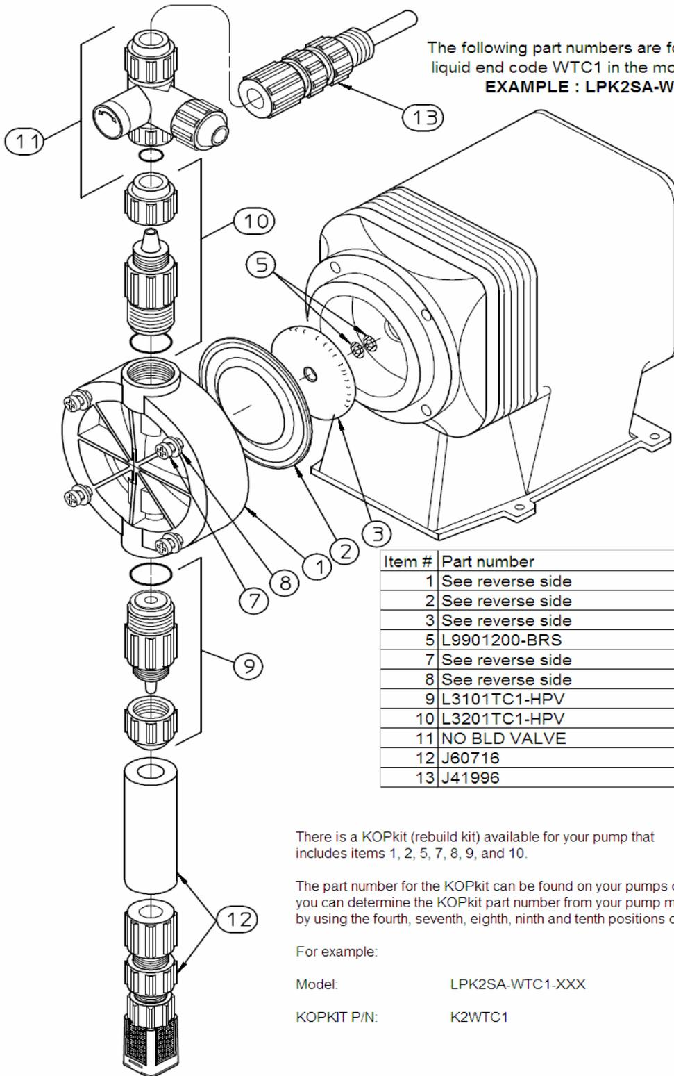
The following part numbers are for pump models with liquid end code WTC1 in the model.
