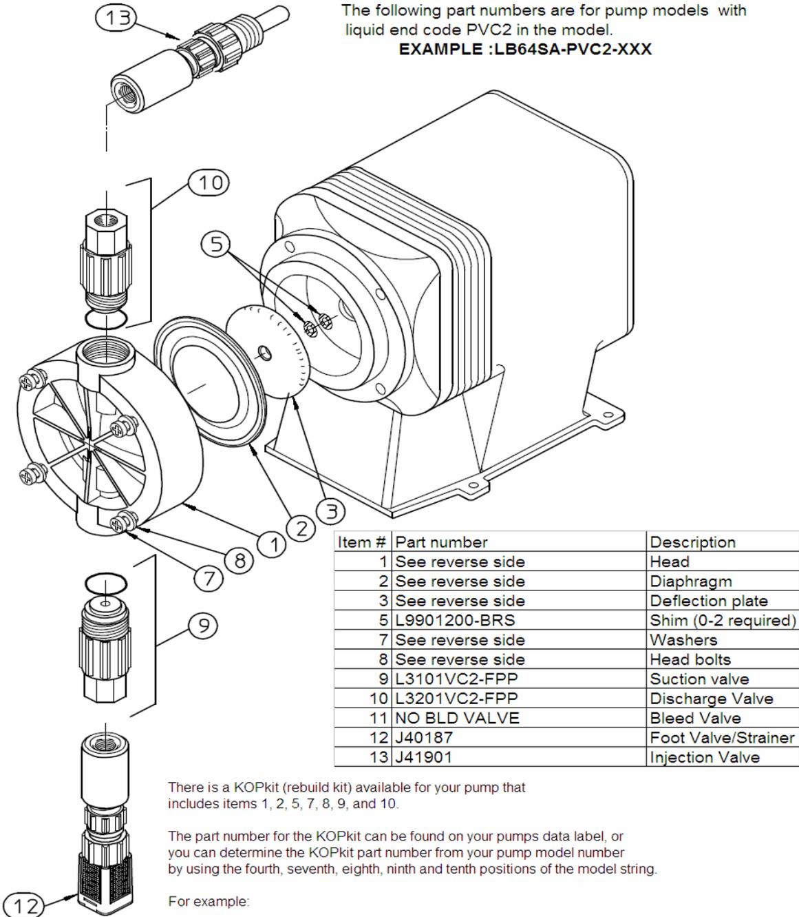
The following part numbers are for pump models with liquid end code PVC2 in the model.
