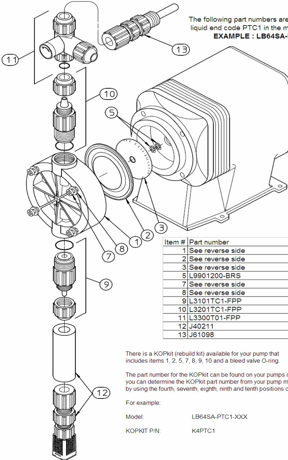
The following part numbers are for pump models with liquid end code PTC1 in the model.
