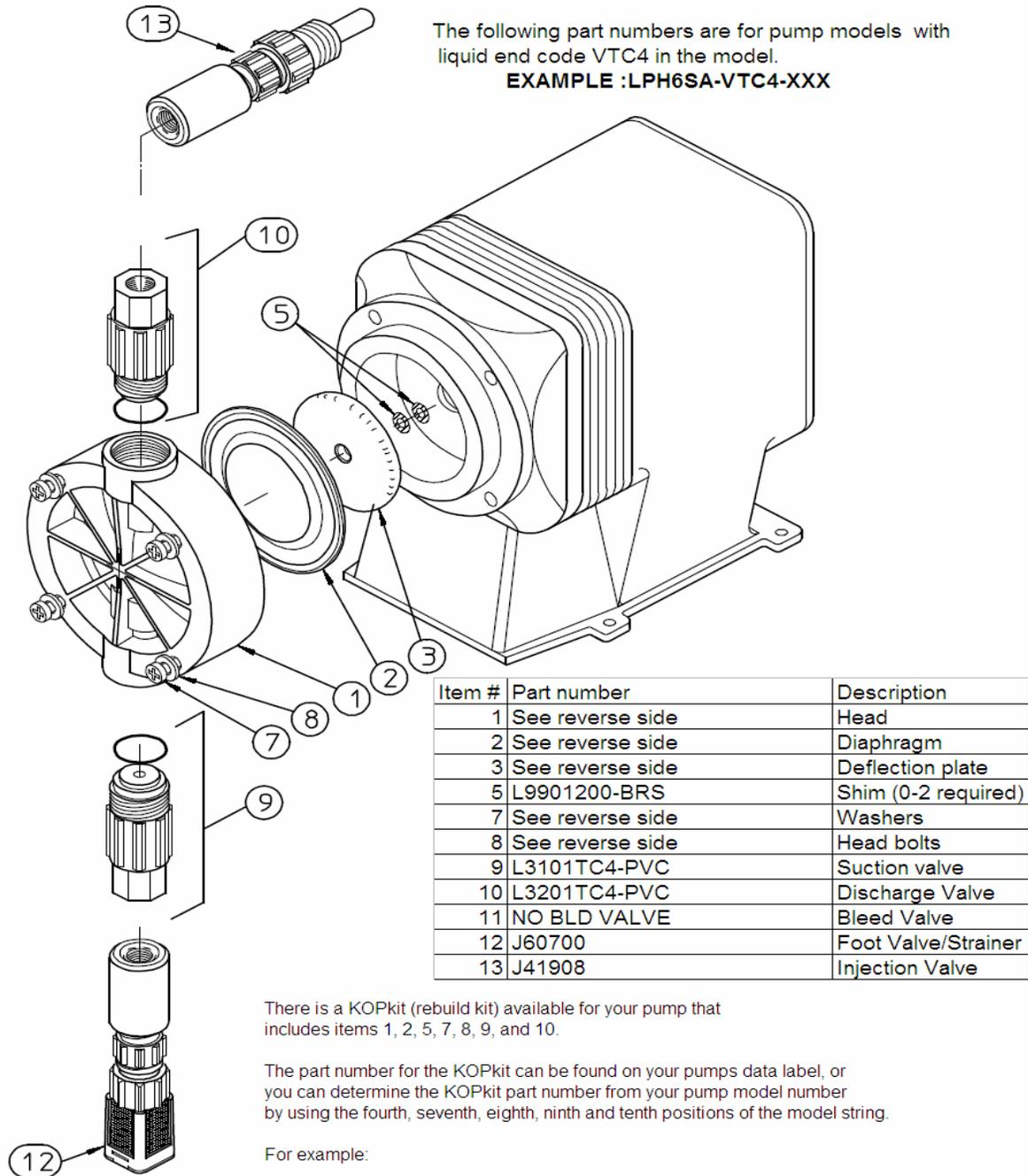
The following part numbers are for pump models with liquid end code VTC4 in the model.
