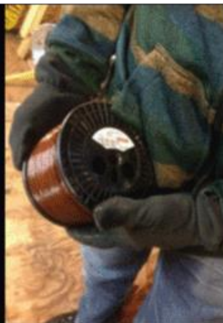
20 GAUGE MAGNET WIRE
