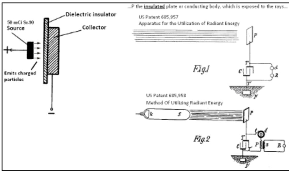
That is essentially Dr. Tesla's radiant energy collector with the insulated, elevated plate horizontal and the charged particles provided by cosmic rays rather than Strontium 90. Note that the plate is not only insulated but insulated with a dielectric, the purpose of which is to separate the charges and keep the collected charges in the conducting metal circuit by preventing them from equalizing with charges in the surrounding air.
